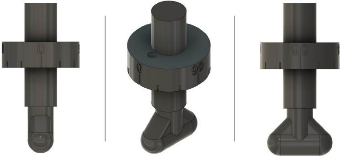
Figure 4.2: CAD model of the capsule prototype design is shown in the front view (left), oblique view (middle), and side view (right).
