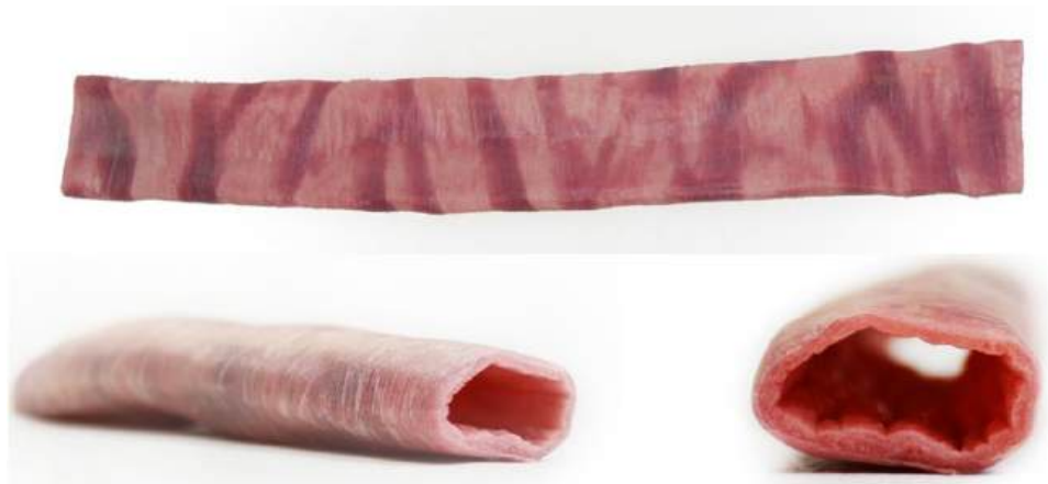
Figure 3.2: A 12-inch synthetic double-layer bowel model from SynDaver was used for experimentation.
