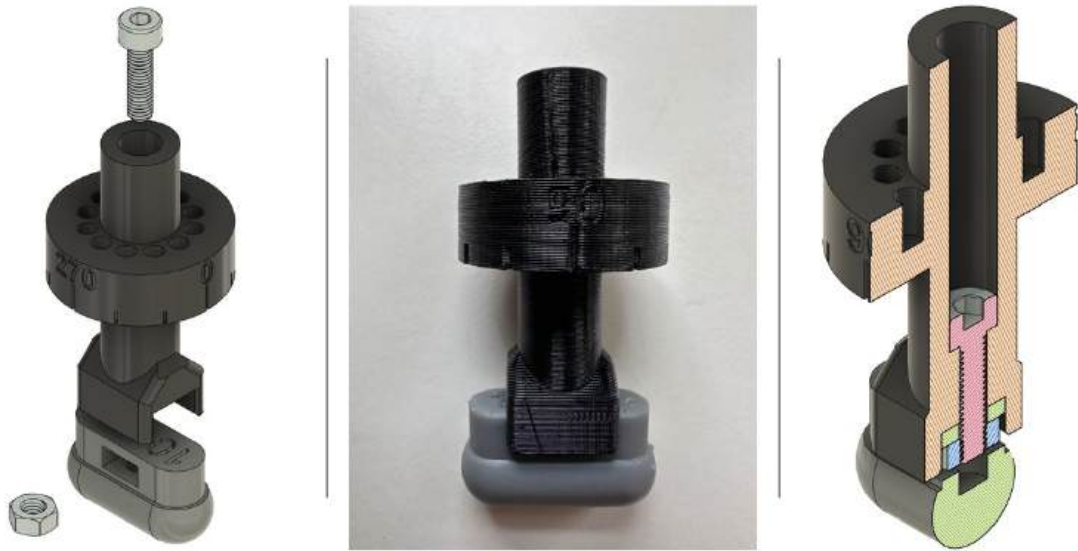
Figure 4.8: Images include the probe holder, schematic drawings in exploded view, and cross-sectional views.
