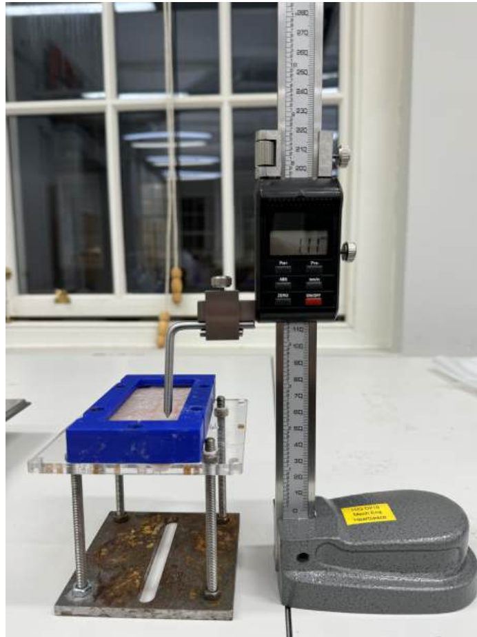
Figure 3.6: Device and setup for measuring tissue thickness.
