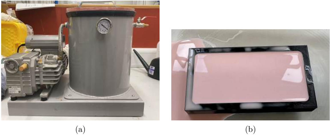
Figure 4.3: (A) Vacuum machine that was used for de-airing. (B) Silicone curing in the mould.
