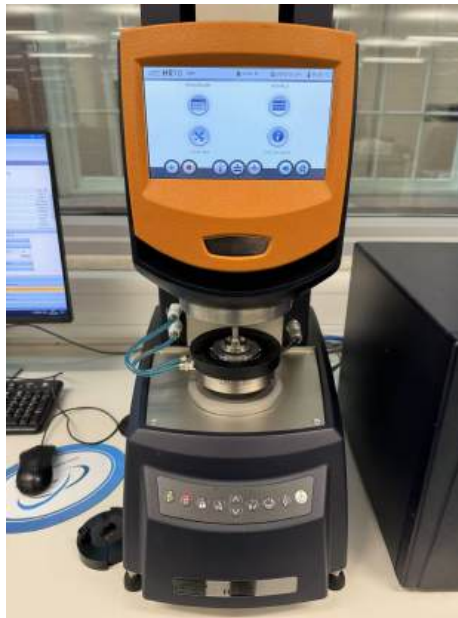
Figure 5.3: Viscosity of each mucus type versus shear rate was measured by using the rheometer.
