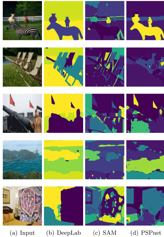
Figure 5.7: Comparison of Segmentation Networks on Manipulated Images, generated by three state-of-art pre-trained image segmentation methods.
