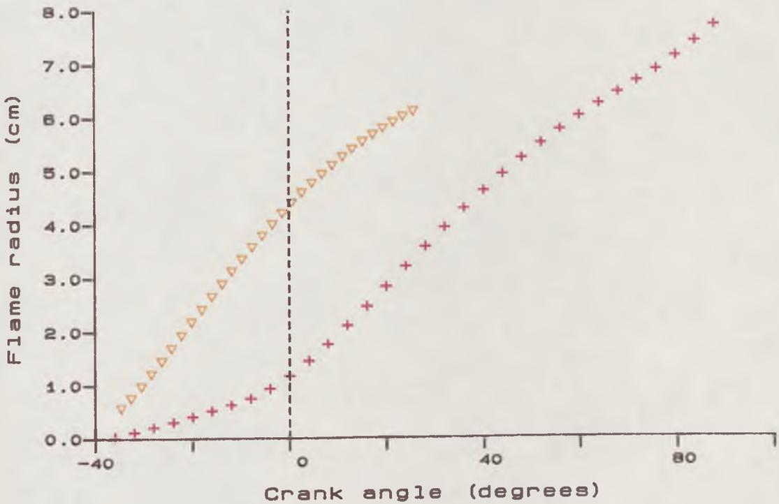
Fig. 5.16 Comparison of Experimental And Predicted Flame Radii
