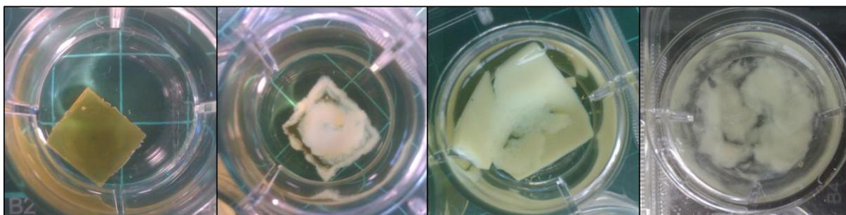
*Figure 10: Swelling and fragmentation of cured PLA samples. The PLA samples rapidly increased in mass, turning opaque and finally undergoing fragmentation. Images taken after 0, 1, 2 and 7 days (left to right).*
