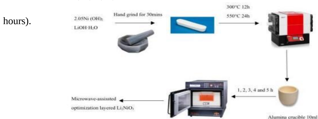
Fig 4.1 Reaction scheme used for the microwave-assisted optimization synthesis of \text{Li}_2\text{NiO}_3 .
