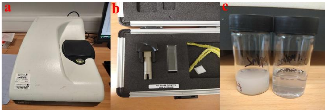
Figure 3.37 - Zetasizer for DLS and Zetapotential Measurements (a), Dip cell and Quartz Cuvette (b), TiFeSi Support in Methanol at 1 \text{ mgml}^{-1} and 0.1 \text{ mgml}^{-1} Concentration (c)
