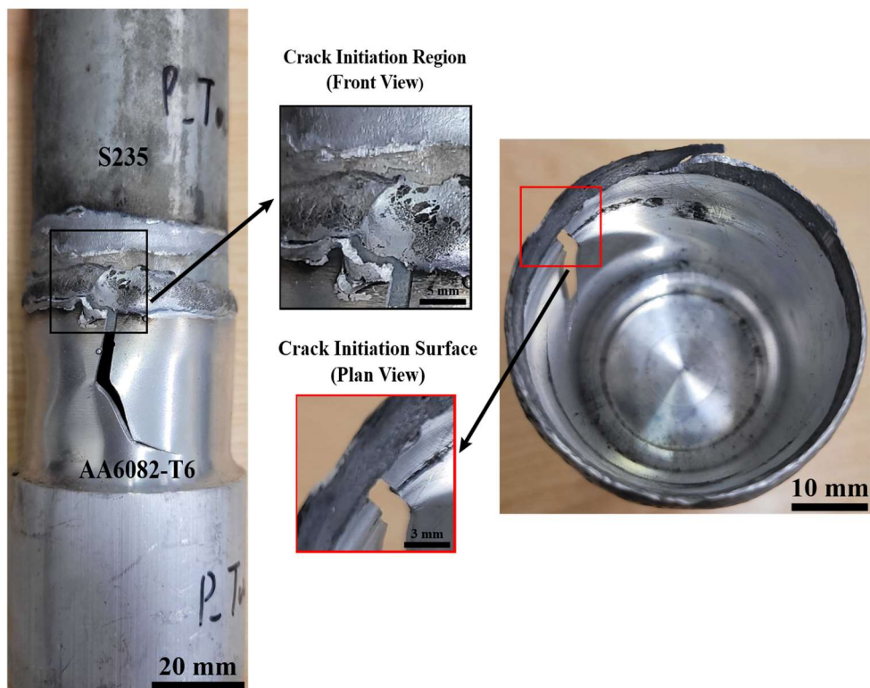
Figure 6.4: Representative crack initiation sites under pure torsional fatigue loading: (a) weld start/stop position, (b) weld toe/root and (c) weld itself.
