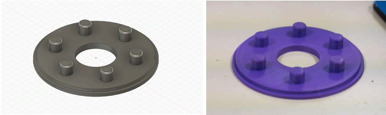
Figure 7. Rendering and physical view of custom well template designed for feeding assay. Designed in Fusion360, sliced in Cura and Printed in PLA+ on an Artillery Sidewinder X1
