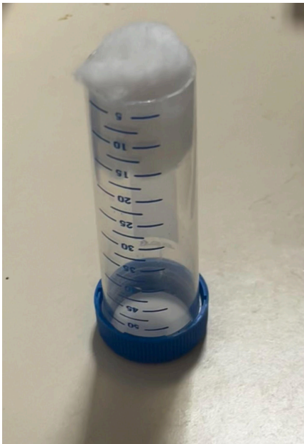
Figure 6. Modified falcon tube used for experimental exposures. The base of each tube was removed and replaced with cotton wool. Exposures were pipetted onto two layers of Whatman 1 filter paper in the lid.
