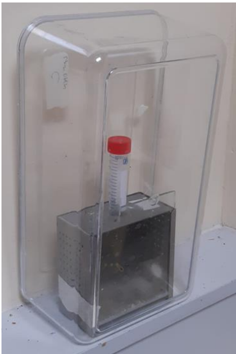
Figure 5.2 – Showing a honeybee cage contained within a plastic box to limit dissipation of pheromone away from cage
