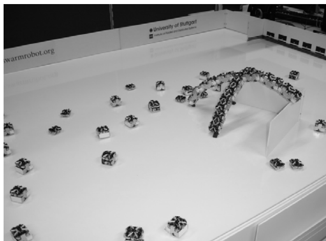
Figure 3.9: An example of swarm robots aggregated together as a multi-modular robot organism [94]
