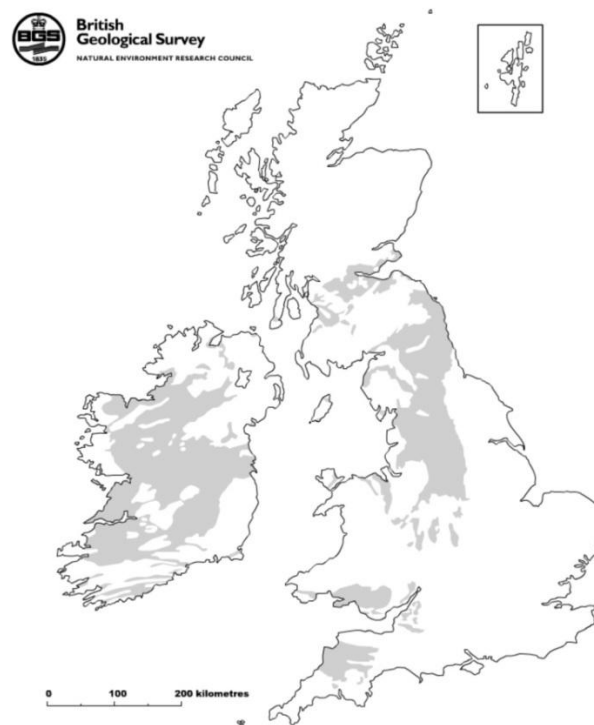
Figure 1 – Outcrops of Carboniferous rocks (shaded areas) in Britain and Eire. Generated from BGS (Stubblefield and Trotter, 1957; 2008).
