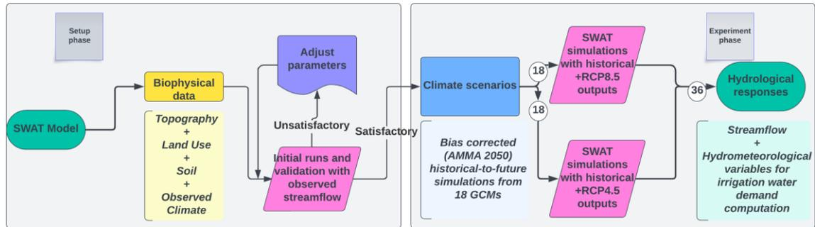
**Figure 4.3 | Experimental framework depicting the connection between the SWAT model and outputs of bias corrected GCMs as well as the variables underlying relationships between drought, irrigation water demand, and supply of water to meet the same.**
