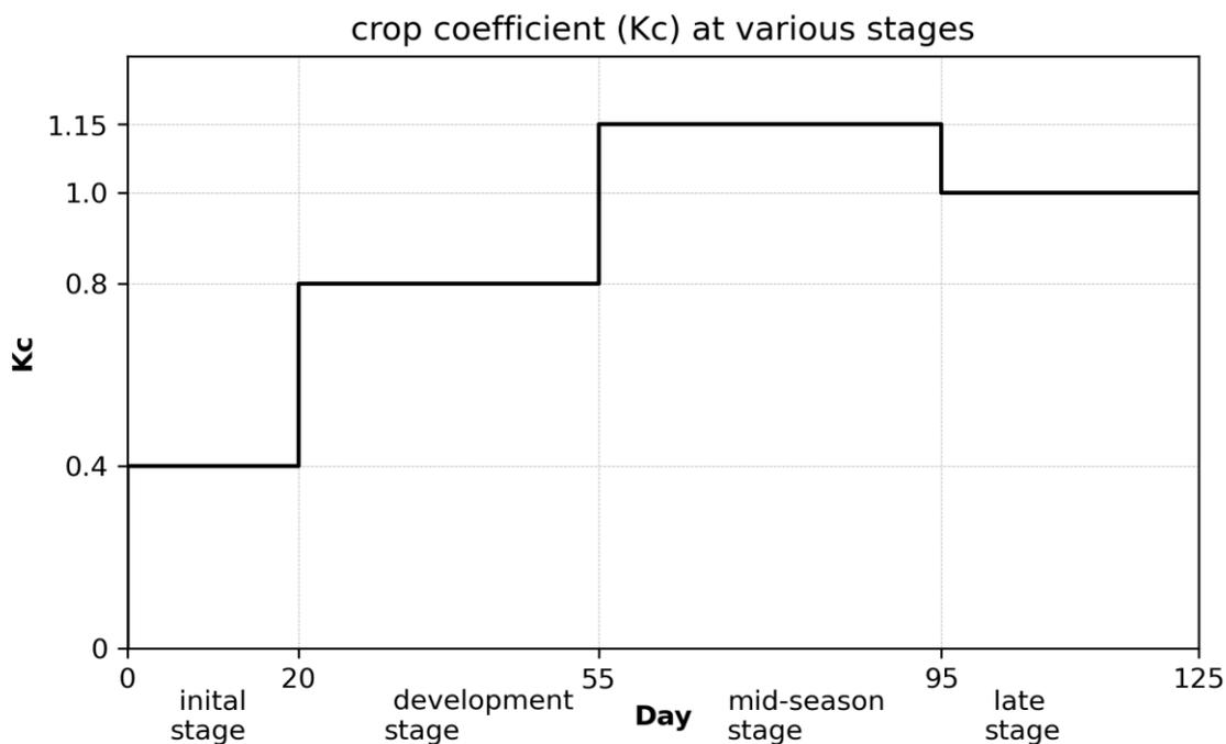
**Figure 4.5 | Crop coefficient (Kc) values for maize at various crop stages from the initial stage to the late stage. This is based on the assumption that the crop has a cycle of 125 days.**
