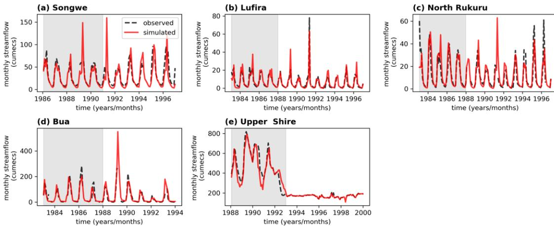
**Figure 4.4 | Simulated and observed streamflow at the most down-stream station for each of the five basins as follows: (a) Songwe at Mwandenga (9B7); (b) Lufira at Ngerenge (9A2); (c) North Rukuru at Mwakimeme (8A5); (d) Bua at S53 Bridge (5C1); (e) Shire River @ Liwonde (1B1). For each plot, the shaded area indicates the calibration period for the corresponding river basin.**
