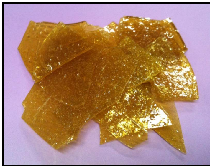
Figure 80: Shellac flakes. These were melted and then used to secure transfer lines to the glass chips during evaluations of bonding agents
