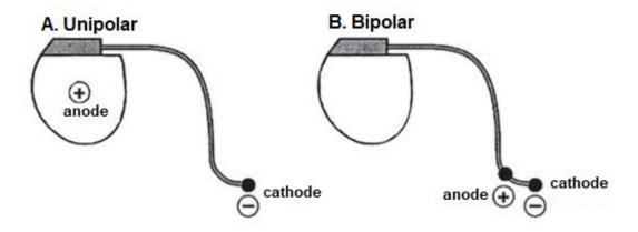
Figure 1.5 (A) Unipolar system; the lead tip is the cathode and the pacemaker is anode, (B) Bipolar system; the lead tip is the cathode and the proximal ring is the anode.
