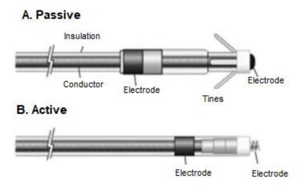
Figure 1.4 (A) Image of passive fixation lead; small fixation tines get tangled in the trabeculations of the heart muscle, (B) Image of active fixation lead; small helix-screwed on the heart muscle
