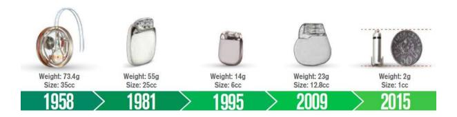
Figure 1.2 The evolution of pacemakers from the 1958 (left) to the present day, showcasing a leadless pacemaker (right) with battery longevity ranging from a few months in early models to over ten years in current models. (Image courtesy of National University Heart Centre Singapore).
