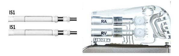
Figure 1.3 Schematic showing IS1 right atrium (RA) lead, IS1 right ventricular (RV) lead aligned before insertion into a pacemaker
