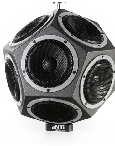
Figure 22: An NTi Audio DS3 Dodecahedron Speaker is suggested as one option for omnidirectional amplification of the logarithmic sweeps. As can be seen in the picture, due to the construction and requirement for the number of speakers for this to be achieved, the size of the speaker drivers are limited, and in turn, the amplitude able to be achieved, especially at lower frequencies, is compromised. From [75] .
