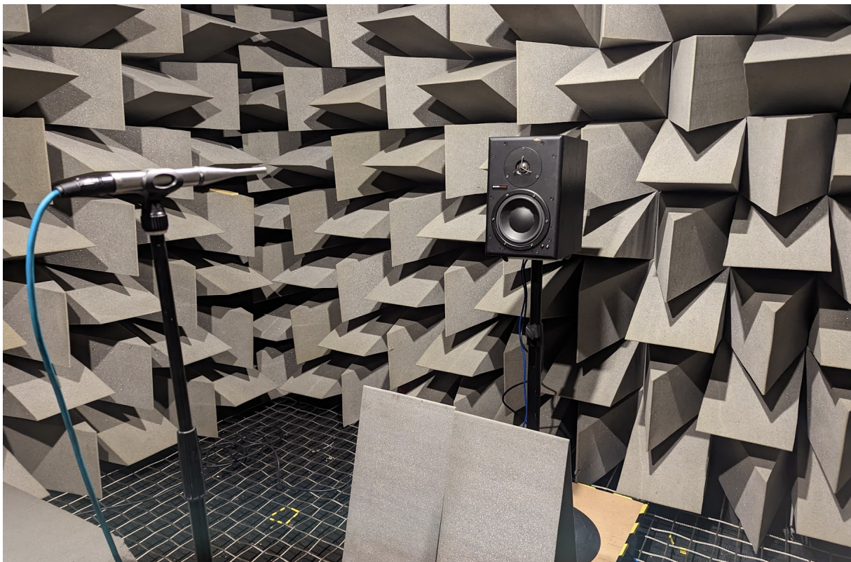
Figure 33: Measurement of the Dynaudio BM6a speaker and recording system in an anechoic chamber
