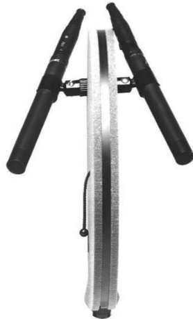
Figure 17: A pair of Omnidirectional condenser microphones baffled by a Jecklin Disc. From [48] .
