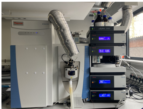
Figure 1.13: Ultimate 3000 UHPLC (Thermo Scientific, USA) and Q Exactive Orbitrap MS (Thermo Fisher Scientific, USA) used for OA analysis at the University of York
