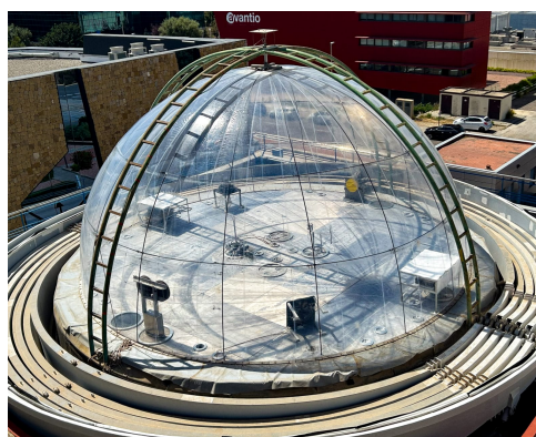
Figure 4.1: 200 m 3 Teflon chamber at the European PHOtoREactor (EUPHORE) facility in Valencia, Spain
