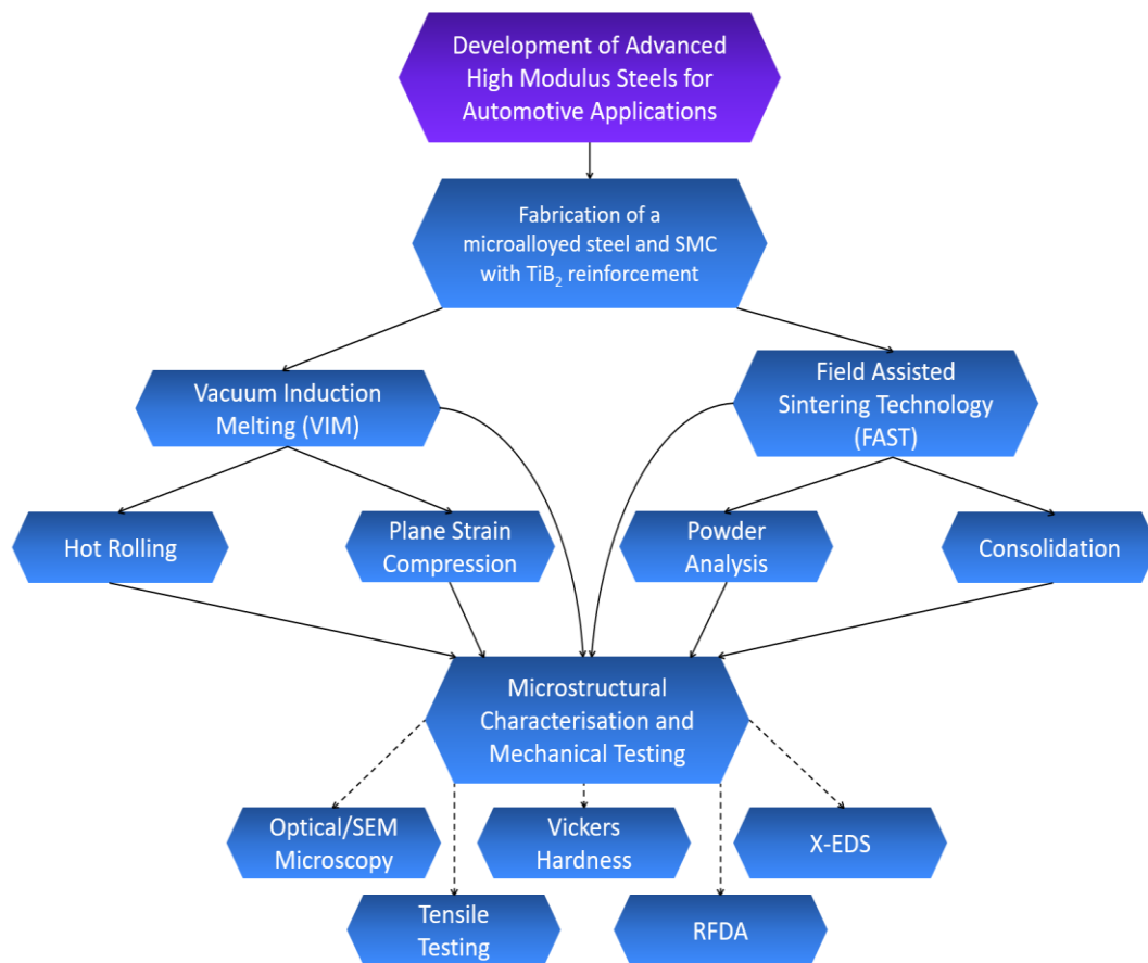
Figure 1: Flow diagram illustrating processing and analysis routes for VIM and FAST
