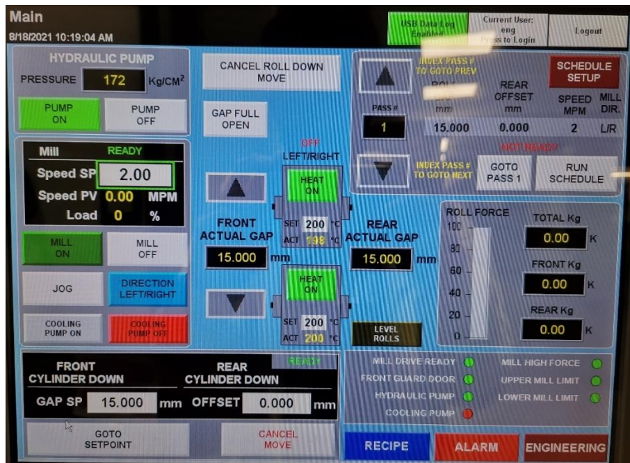
Figure 19: Live screen view on the FENN mill during hot rolling, illustrating various input/output variables and information on the reverse rollers
