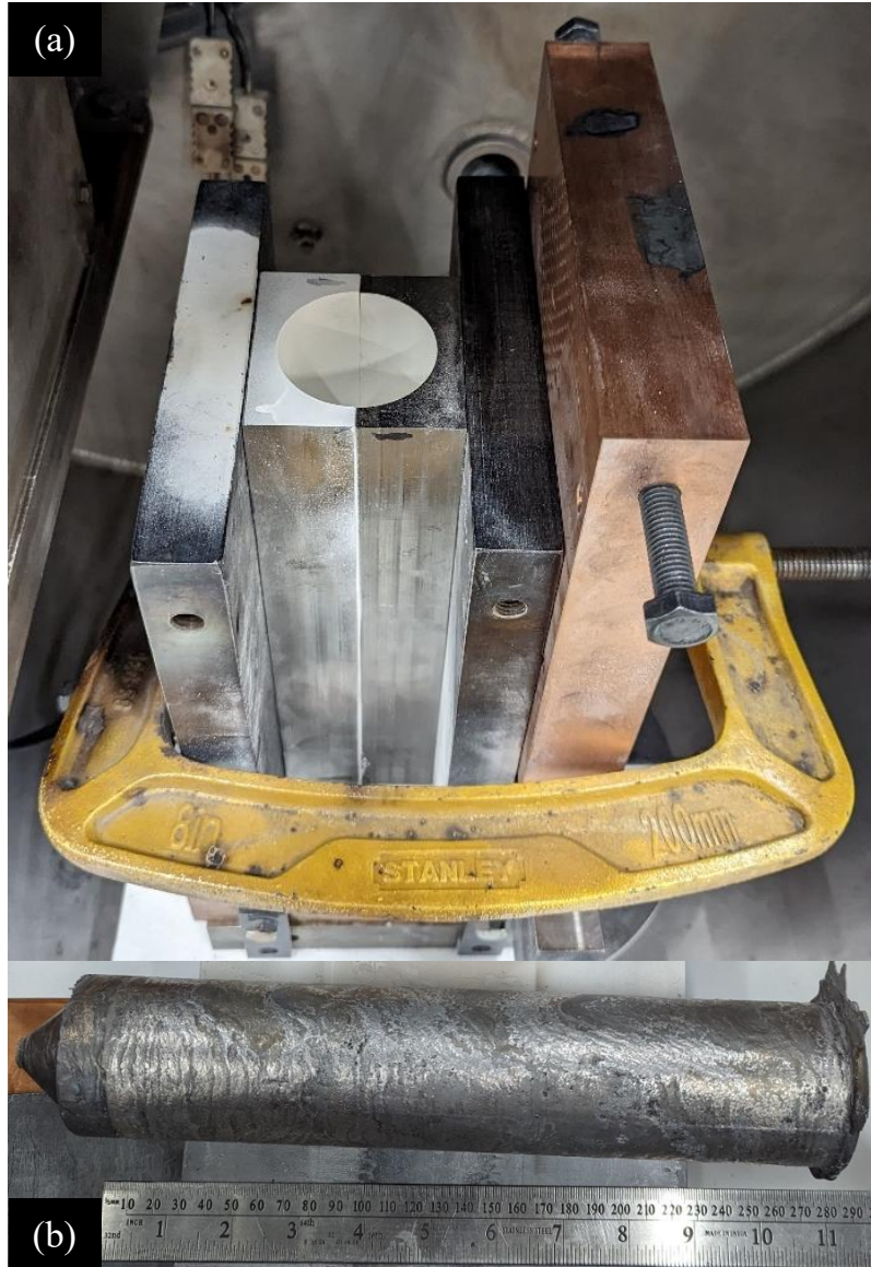
Figure 25: (a) VIM mould assembly for casting the cylindrical MA steel bar and (b) as-cast MA steel bar with a cone-shaped end for atomisation
