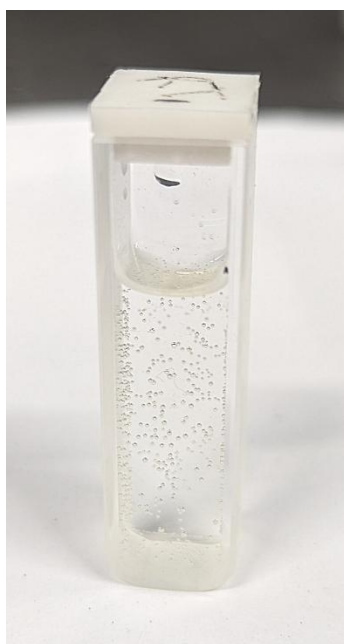
Figure 4.26. Room temperature sample in an unstoppered cuvette after 1 day. Large numbers of bubbles, presumably HCl, have nucleated in the solution.
