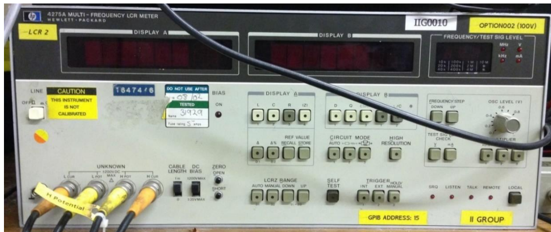
Figure 3.7 Front of HP 4275A LCR meter used in CV set up
