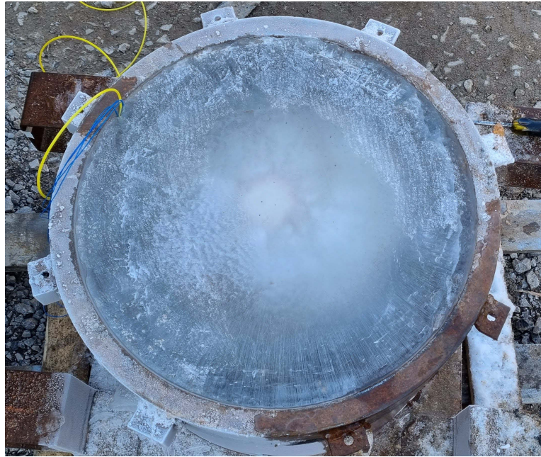
Figure 6.11: Photo of the soil container filled with ice prior to the test, showing the charge in the centre (white disc in orange charge case).
