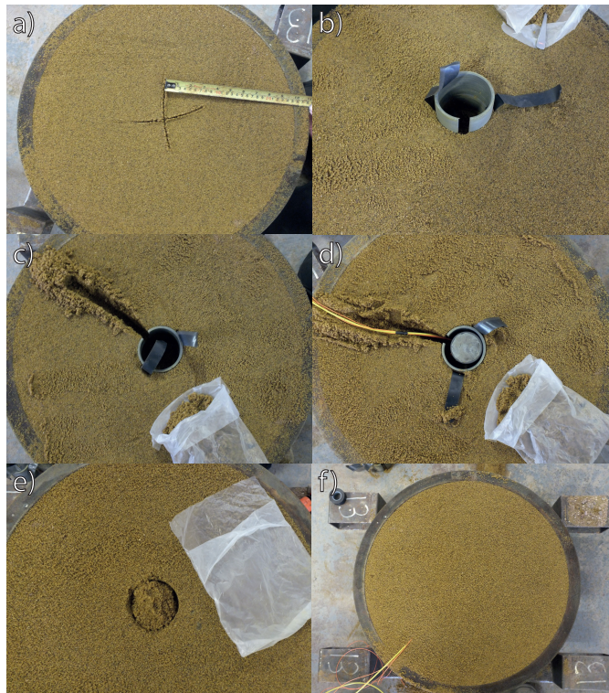
Figure 3.5: Photos showing the method for placing a charge in a pre-prepared sand bin whilst minimising the degree of disruption to the geotechnical parameters.
