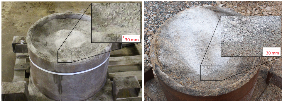
(a) Post test photo from Shot003, testing with unfrozen LB sand in § 7 (b) Post test photo from Shot024 with frozen LB sand
