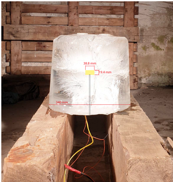
Figure 6.8: Image of an ice block pre-test. The block is supported on two timber stands, with the detonator (yellow tube) and a camera trigger wire (orange) inserted through a long hole to the charge from the lower face (indicated by the dashed lines).
