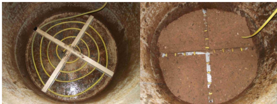
Figure 3.4: Photos showing the position of the saturation hose at the base of a soil bin. The bin is filled and compacted prior to saturation (Clarke et al. 2014).
