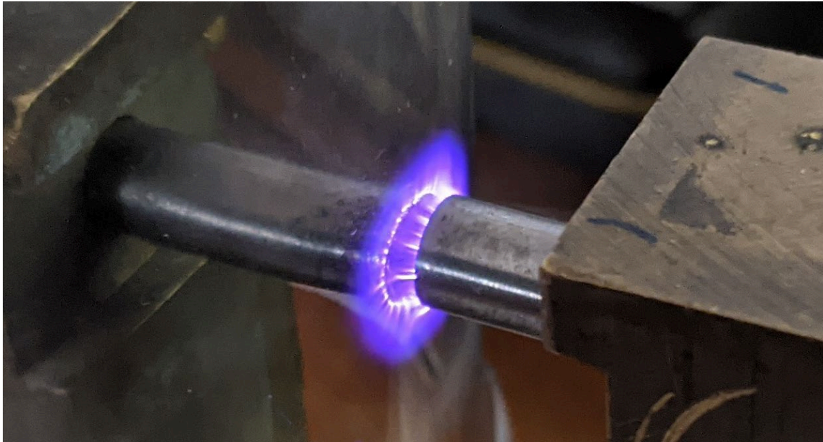
Fig. 1.2 Photograph of DBD plasma in air (photograph by author)
