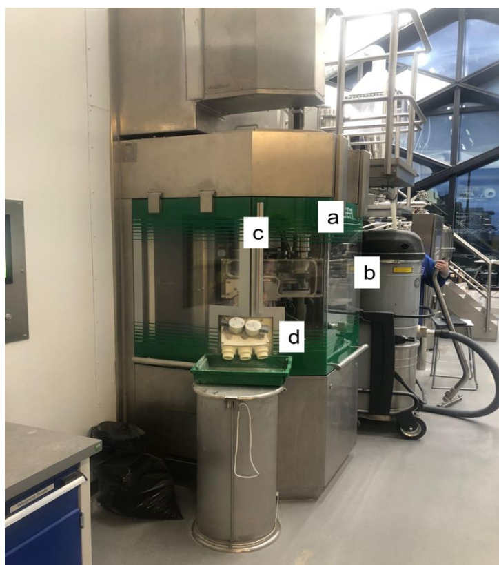
Figure 3.12 Rotary tablet press: (a) Feeding point, (b) Feeding frame, (c) Feeding paddles and (d) Ejection point.
