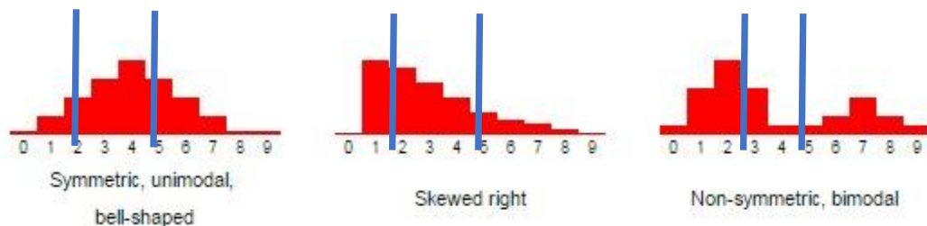
Figure 4.20 Typical forms of the granule particle size distribution.
