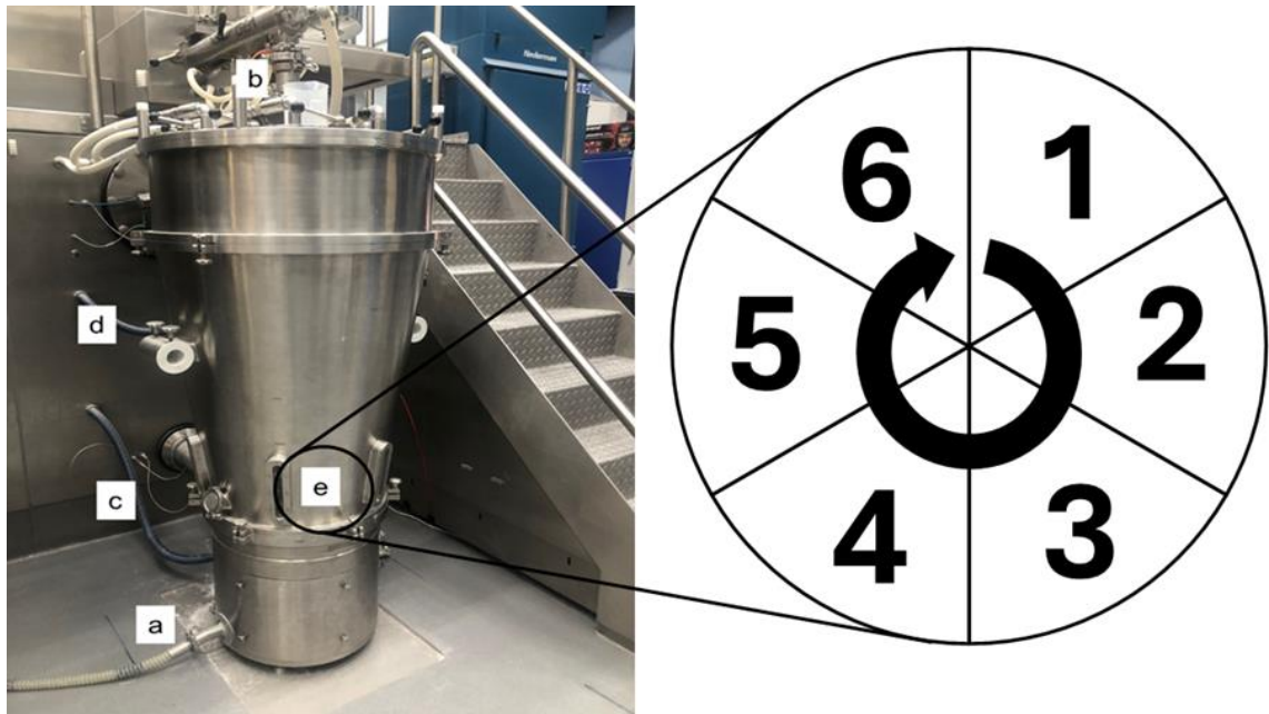
Figure 3.9 DiPP Fluidised bed drier: (a) Dried granule outlet, (b) Wet granule inlet, (c) Drying air inlet tube, (d) Drying air outlet tube and (e) 6 segmented drying cells.
