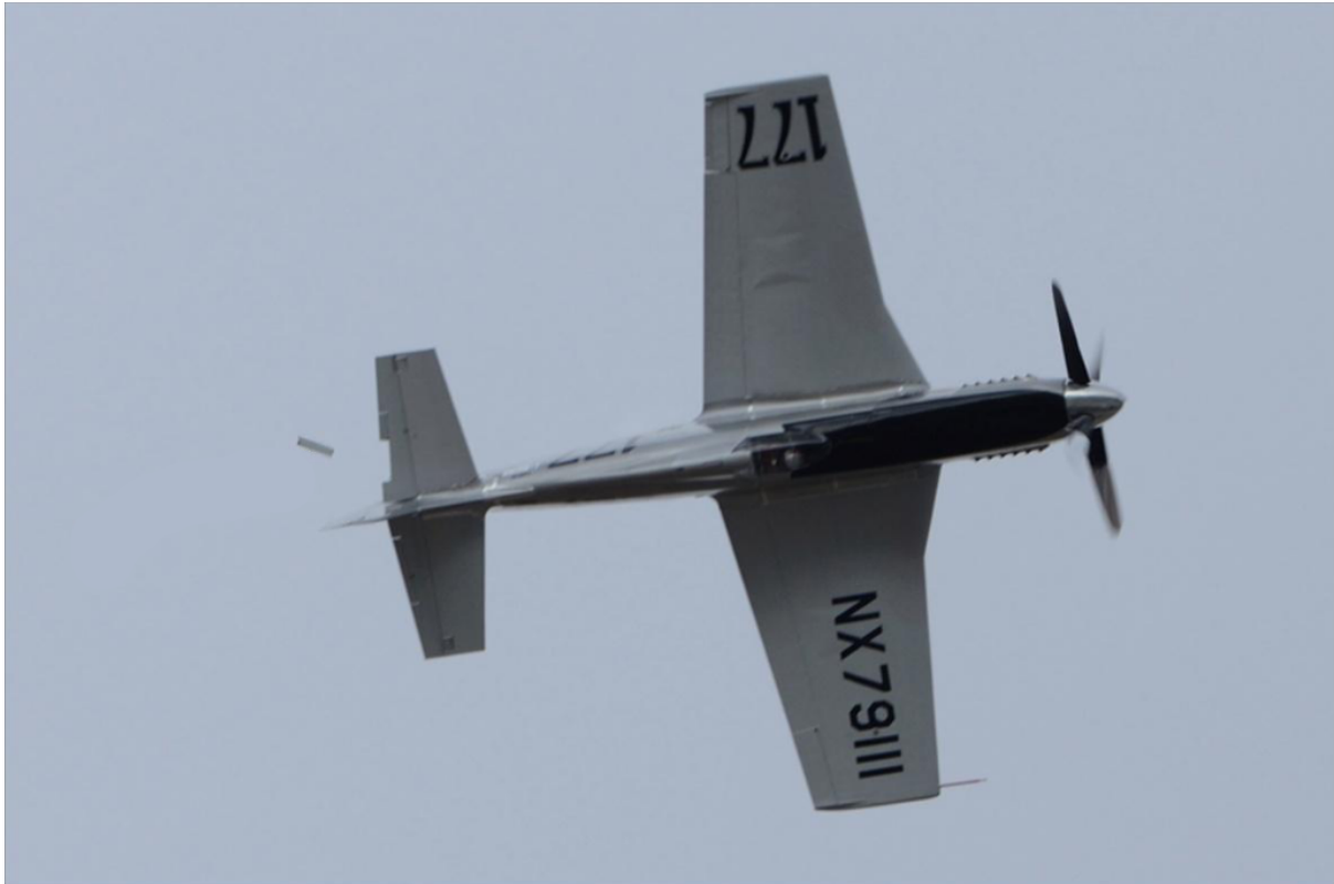
Figure 2.3: P-51D Mustang, The Galloping Ghost , lost its elevator trim tabs during Reno Air Races [17]
