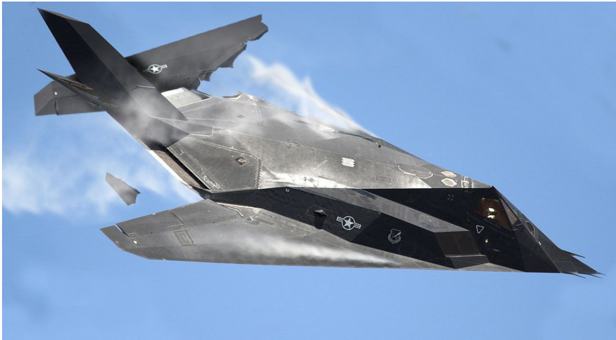
Figure 2.1: The damaged F-117A before crash at Chesapeake Air Show [14]
