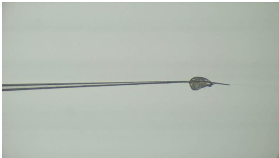
Figure 115. Optical microscope image of the Nafion – Pt(B)/CNT on CFM after measurements were concluded. It was evident that cells had adhered to the quartz outer capillary of the CFM during the measurements.
