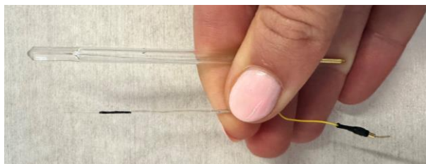
Figure 9. A photograph depicting two different varieties of microelectrode (top) platinum microelectrode, (bottom) CFM – both microelectrodes have a 15 \mu\text{m} active surface area when unmodified.
