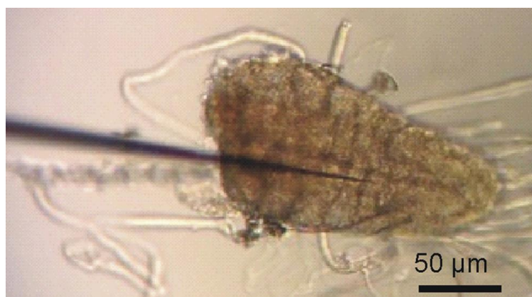
Figure 3. Carbon nanopipettes achieve high spatial resolution in vivo measurements in Drosophila , as shown by the Venton group. 38
