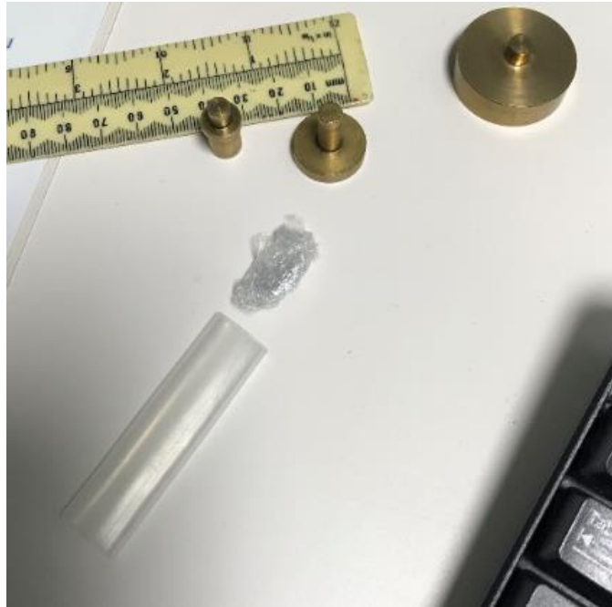
Figure A.1.2. – Plastic tube, nylon foil, and different size chucks (sample holders).
