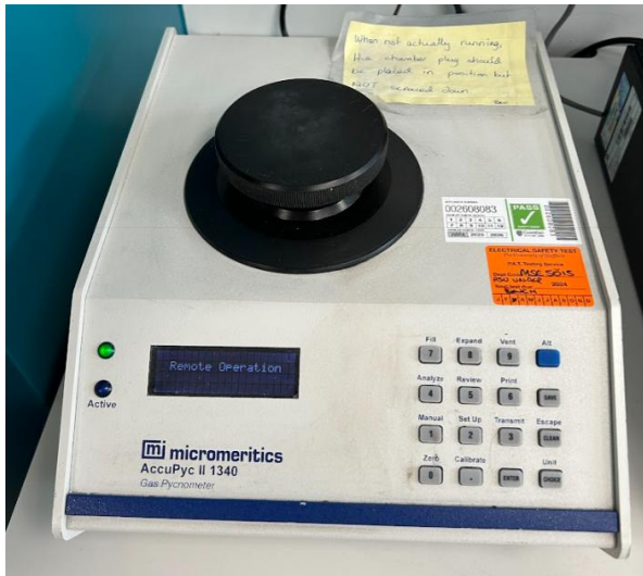
Figure 3.12: Image of Accupyc II 1340 (Supplier: Micromeritics) used for analysis of primary particle true density
