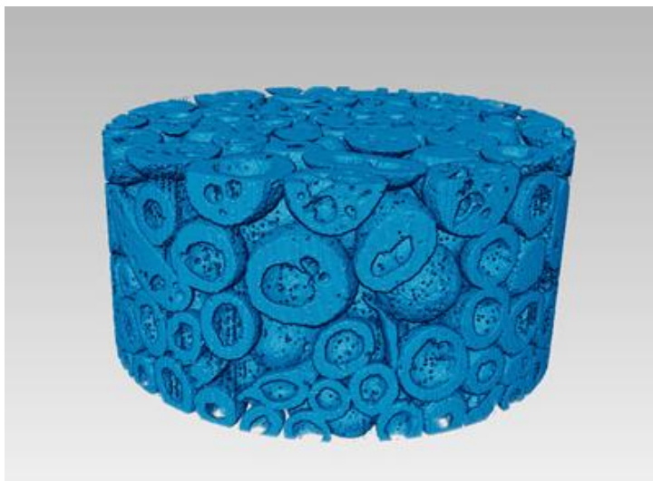
Figure 6.24: Reconstructed 3D render of the XRCT data, where machine learning software (iLastik) was used to identify the regions of solid or air after training of a bed of coagglomerates (Will Dawson, UCL)
