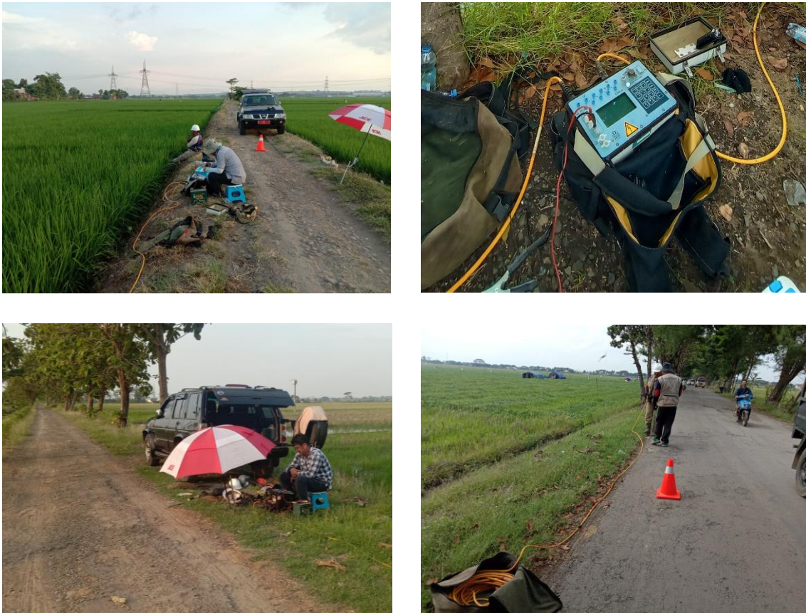
Figure 3.11 Geoelectric measurement activities in the study area
