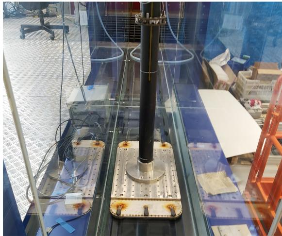
Figure 4.7: Metal baseplate with suction cups used to secure the structure to the wave tank. The photo was taken before the tank was filled with water.
