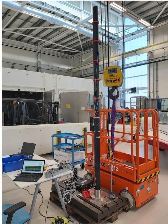
Figure 4.3: The monopile structure before it was placed within the wave tank. The fixed metal base and crane used to load variable masses to the top of the structure can be seen.
