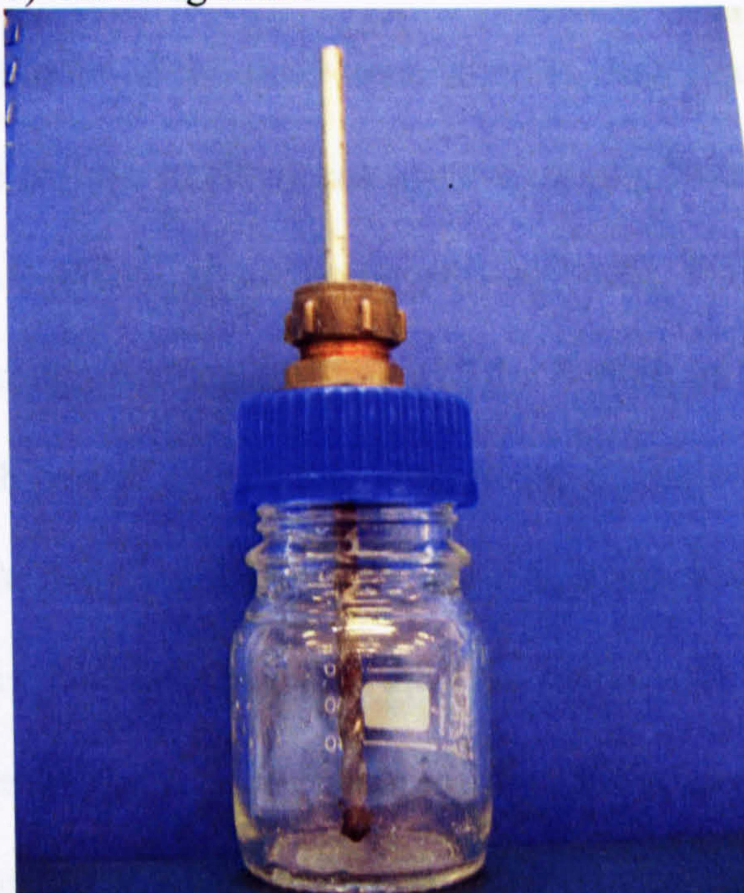
b) Cracking bottle
