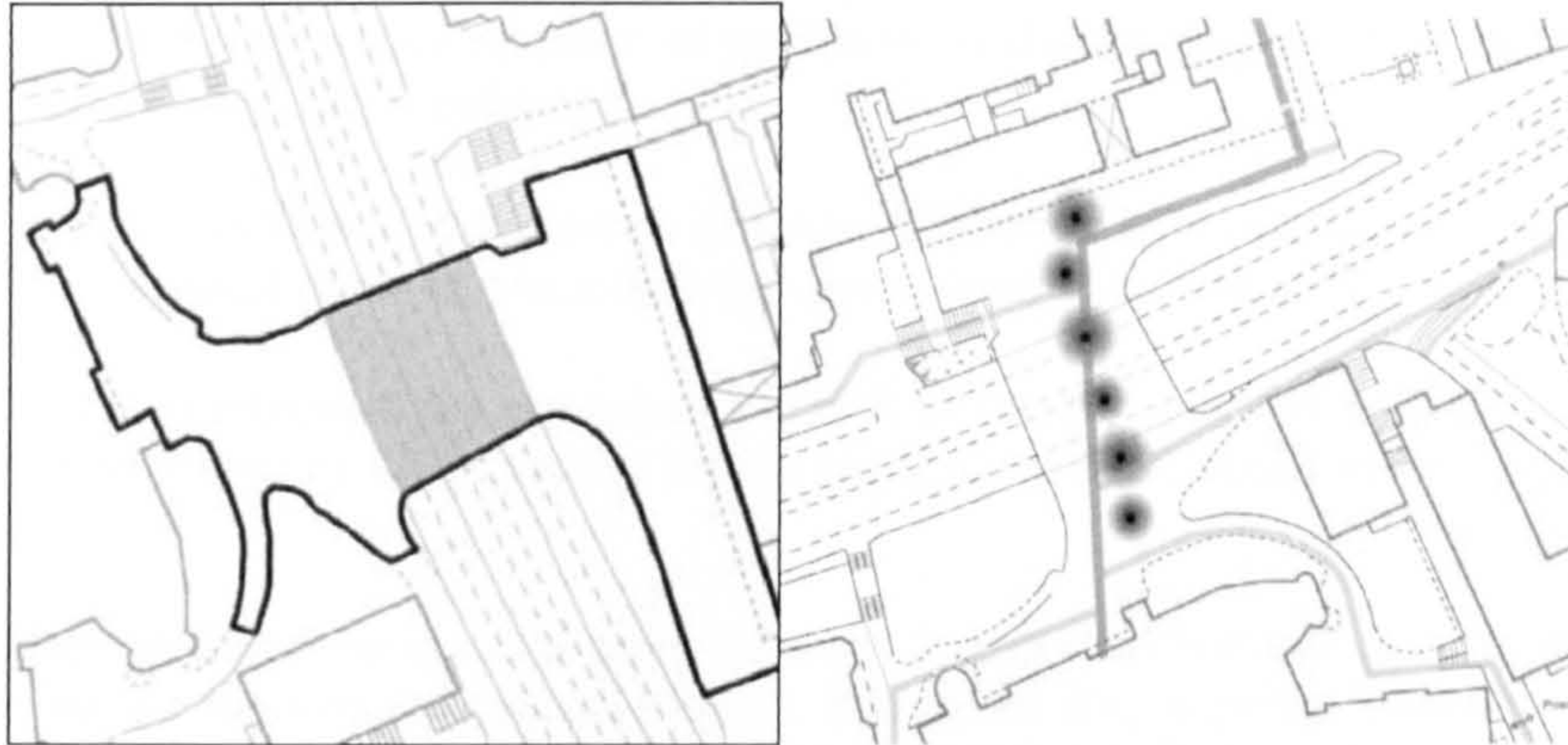
Figure 68: Topology of place and topology of IT in the solutions: first picture is the enclosure to the Interactive games, and the second represents the transmitters (dots) along the paths (pink and yellow lines), in the Bluetooth Advertisement Solution.
