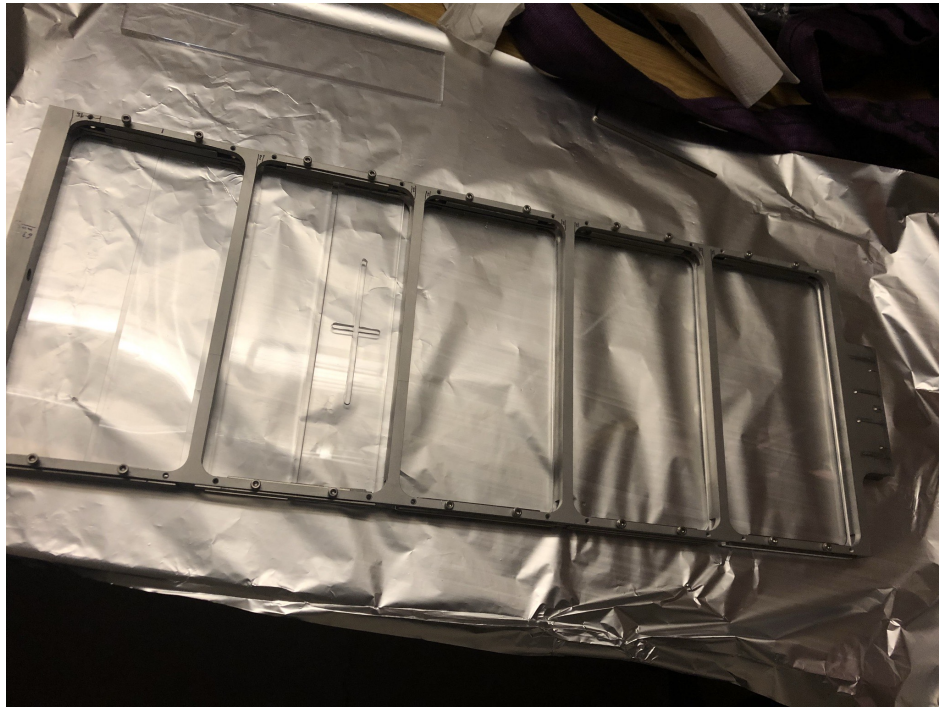
Figure 3.4: The S8 scintillator ladder capable of holding up to 10 scintillating paddles of varying thickness and type.
