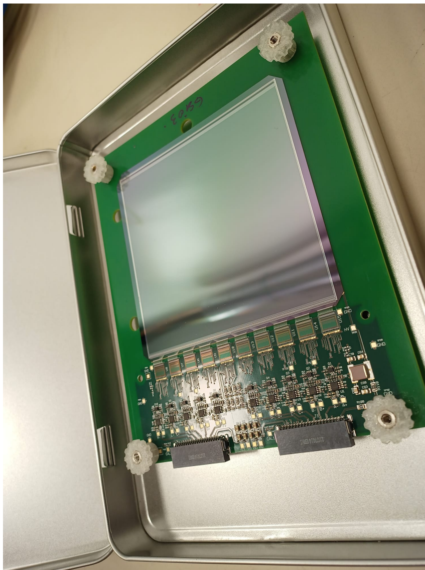
Figure 8.4: Front side of the first R3B FOOT detector. Here all 10 ASICs are visible each connected to 64 strips.
