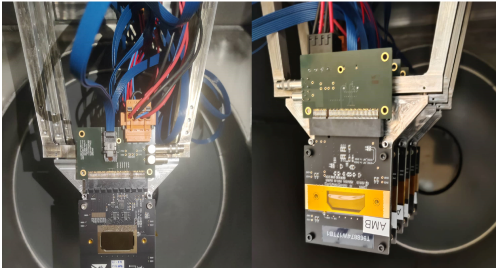
Figure 8.11: The left image shows the back of the SCC telescope and the right the front with respect to the beam. The detectors are placed inside the unified tracking station chamber provided by the AMBER collaboration.
