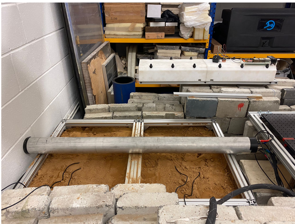
Figure 6.12: Detector in aluminium tube housing.
