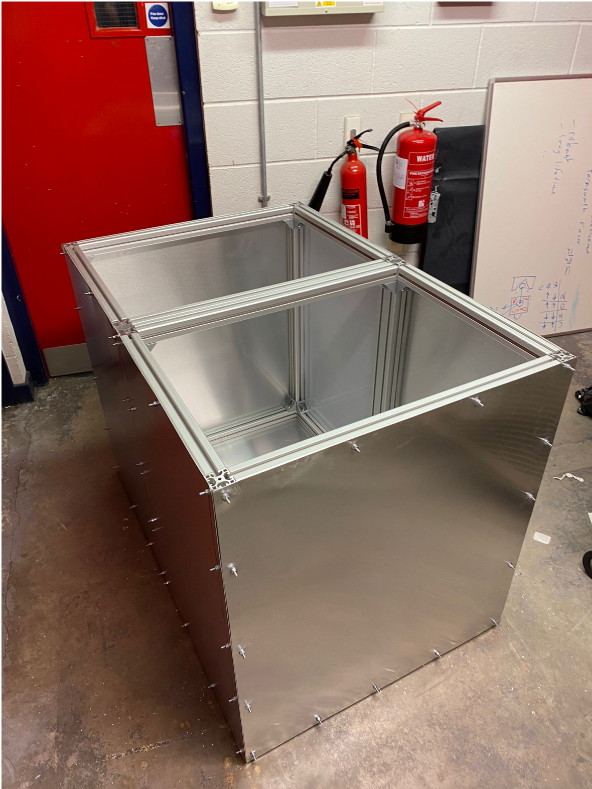
Figure 6.18: Aluminium box constructed to hold variable water content sand volume.
