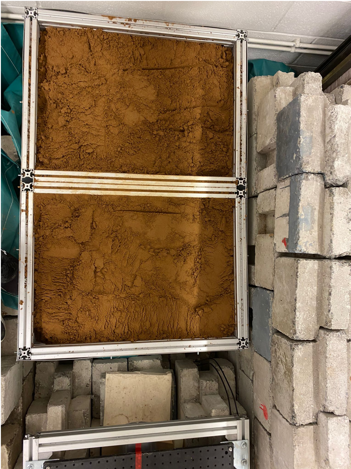
Figure 6.20: Filled aluminium box containing over 1.2 tonnes of builders sand.
