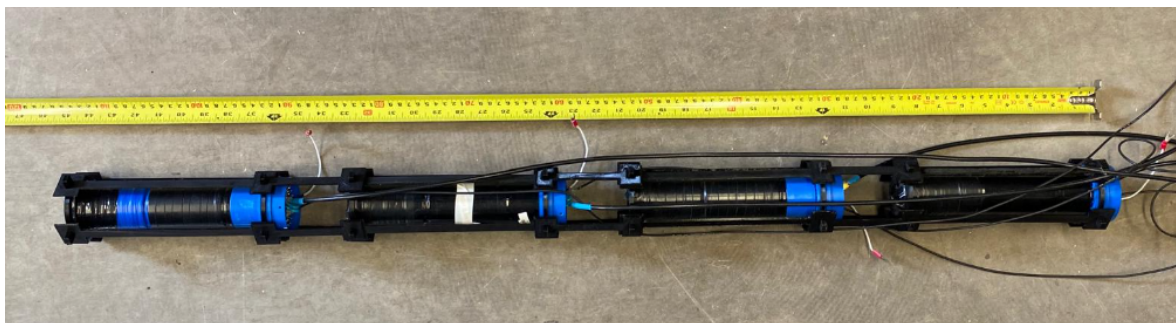
Figure 6.11: Four-detector system. Each detector held in position with lightweight 3-D printed clips ready for housing in aluminium tube.
