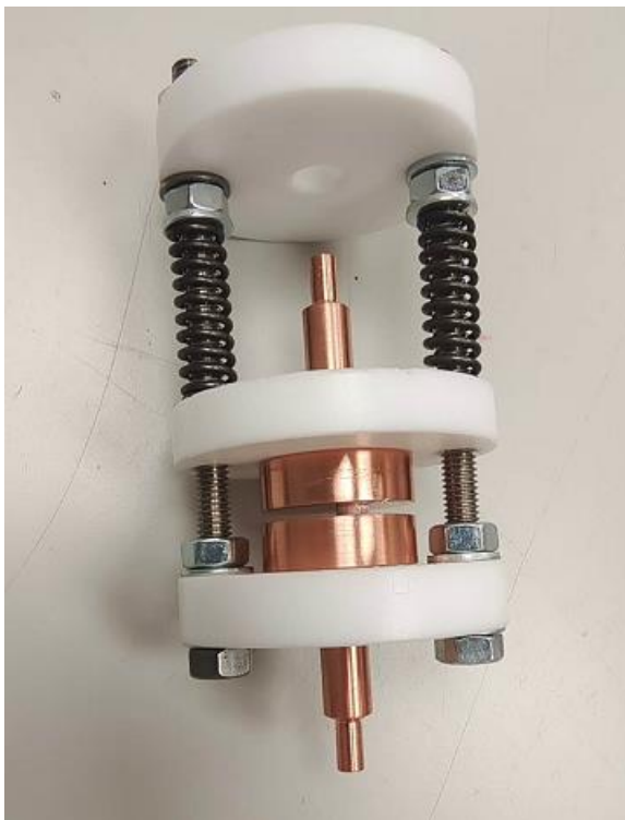
Figure 3.2 Digital photograph of the pellet sample testing cell with two plate electrodes.
