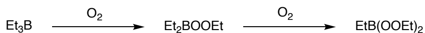
Scheme 31. Reaction of Et 3 B with two moles of O 2 to give the diperoxide EtB(OOEt) 2 .
