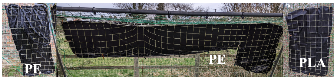
Fig. 3.3. Large sheets of PE and PLA mulches cut from the purchased mulching materials were hung outside to naturally weather from 3 rd April in 2022 to 2 nd August in 2023.
