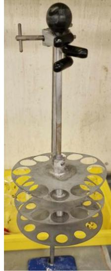
**Figure 3-5** – Small steel carousel used for the fibre analysis acid step.
