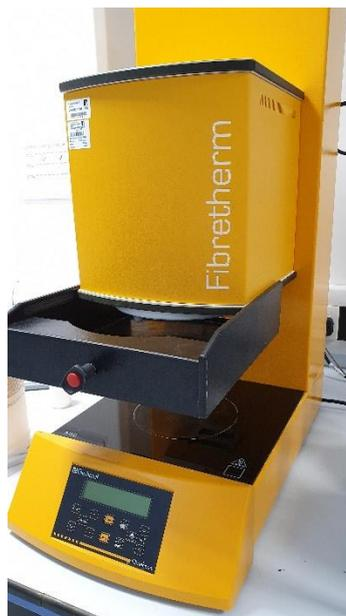
**Figure 3-2** – Image of the Fibretherm equipment used for fibre analysis.
