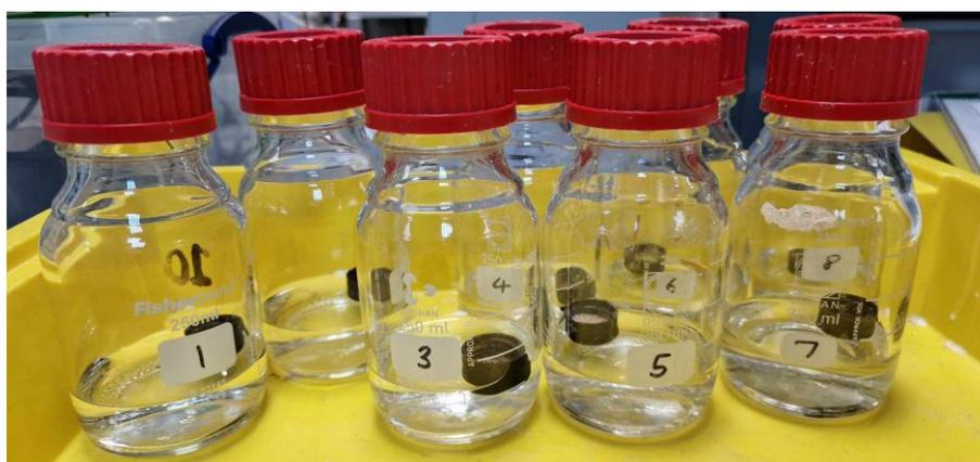
**Figure 3-14** - Batch set-up of ammonia adsorption tests.
