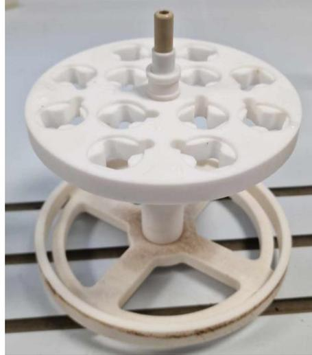
**Figure 3-4** - Carousel used within the Fibretherm equipment for fibre analysis.
