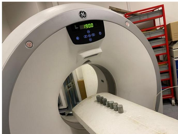
**Figure 3-5.** Wolfson CT Scanner with seven core plugs of ENAP2 set.
