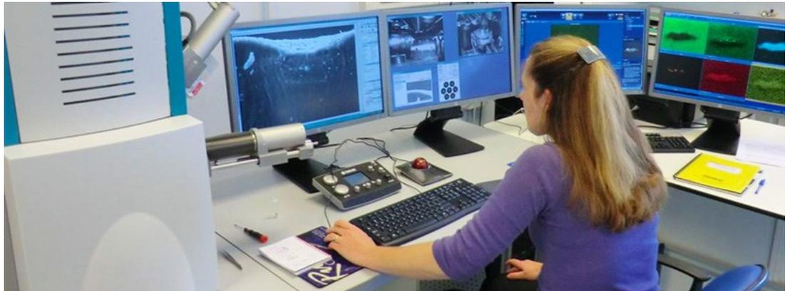
**Figure 3-8.** Scanning electron microscopy model Tescan VEGA3 XM consists of a tungsten source machine with a large chamber and high sample throughput, equipped with X-max 150 Energy Dispersive X-ray spectroscopy (EDS) and Aztec 3.3 software. Also RGB filtered cold-cathode (CL) system (reference photograph from TARR, 2023).
