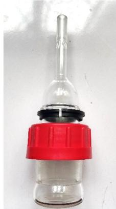
**Figure 3-28.** Custom-made sample tube vessel for BET technique in Wolfson laboratory.
