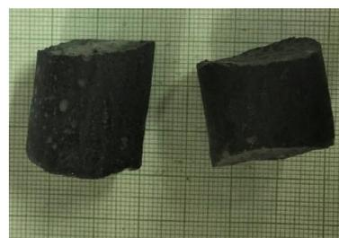
**Figure 3-1.** Sample ENAP1-9 was classified as accepted (left), and sample ENAP1-10 was classified as rejected (right) before core preservation—pictures supplied by ENAP.
