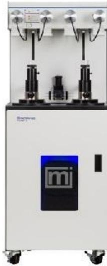
**Figure 3-17.** Micromeritics Autopore IV series model (AZO materials, 2023).
