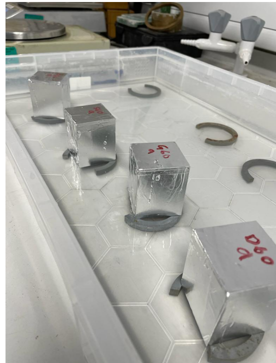
(b) Procedure of the water absorption.
