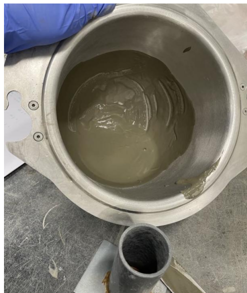
(b) Resulting paste to be poured into cylindrical mould.
