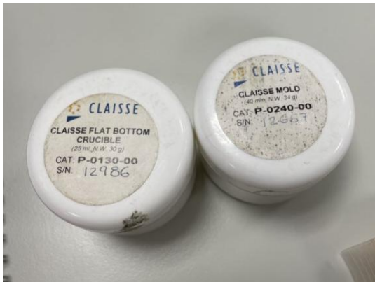
(a) Crucible and base plate use for fuse bead preparation
