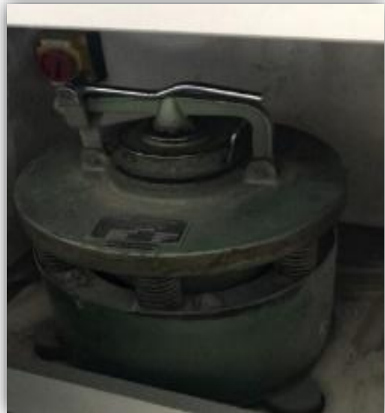
(b) Causes vibration to break the QDs in finer powder
