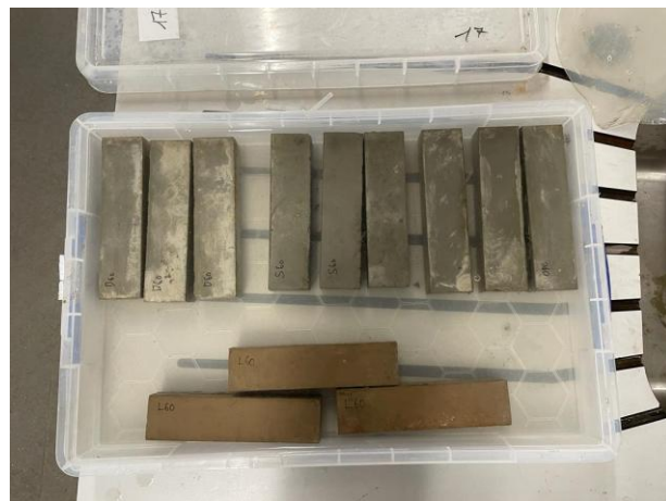
(b): Curing in lime saturated water
