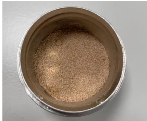
(b) 10g flux mixed with 1g of QD sample
