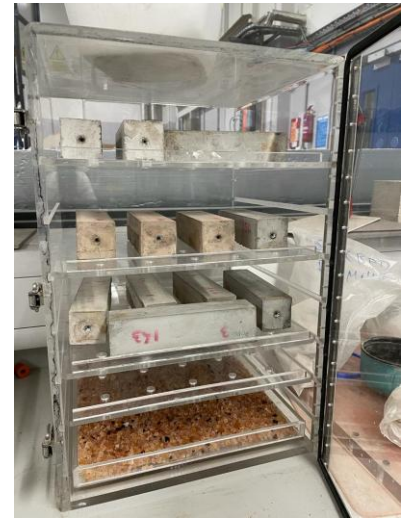
(c) Samples cooled in desiccator.
