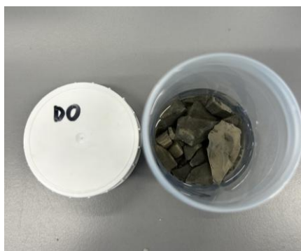
(c) Arresting hydration in acetone solution
