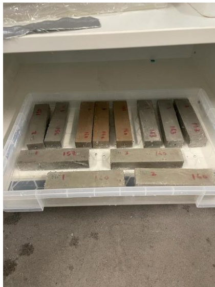
(d) Samples immersed in water for 48hrs
