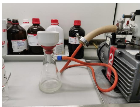
(f): Image of filter, conical flask, and vacuum pump
