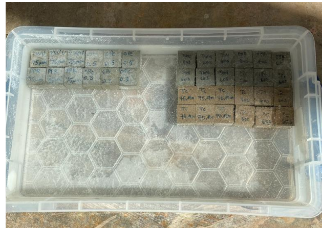
(b) Samples cured for 7 and 28 days.
