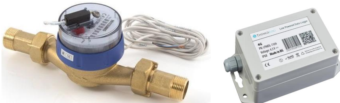
Figure 6.9: Equipment Used for Household Smart Metering (a) BMeters GSD8-I (b) ThingsLog 4G Data Logger
