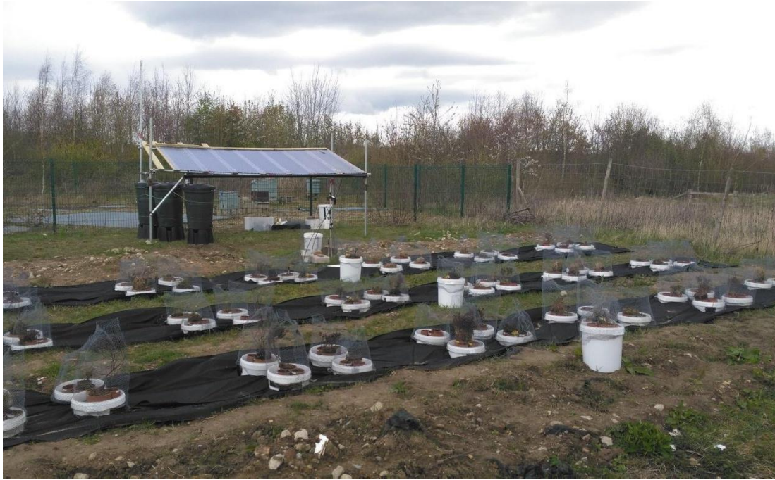
Figure 3.10 Overview of the mesocosm site (referred to as Hes East) at the University of York Heslington East campus, including the on-site rain collection system. Rainwater is delivered to 80 L water storage butts where water is stored until required. 80 L water storage butts where water is stored until required.
