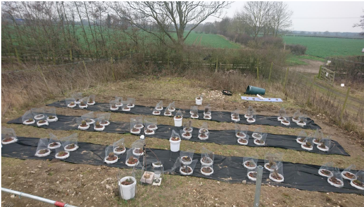
Figure 3.12 Buried mesocosms in purpose dug trenches at the Heslington East (University of York) mesocosm site. Image was taken shortly after installation from the top of the rain collection system. In the centre bottom of the image, the weather station can be seen. The buckets on the soil surface are for soil temperature comparisons.
