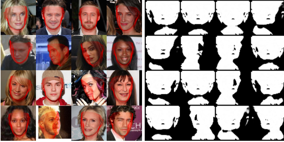
Figure 5.11. Qualitative Results of the Visibility Regressor. The left grids of images show the input face images with the overlaid 3D face shapes rendered using the estimated shape and pose. The right grid displays the corresponding visibility masks predicted by the visibility neural field.
