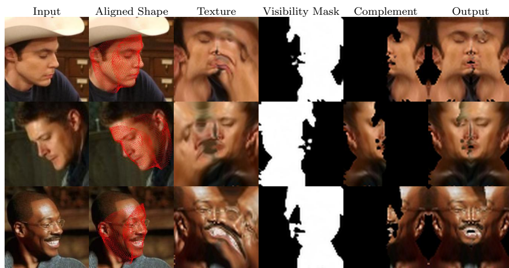
Figure 5.7. More examples for our UV completion. From left to right: input image; alignment shape; re-sample images; visibility masks; Complements used to fill in invisible areas; final re-sampled textures.
