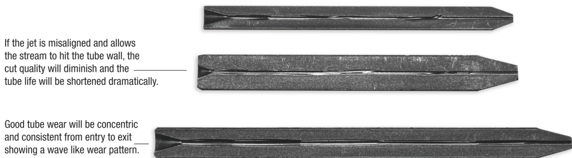
Figure 2.4: Longitudinally sectioned mixing tubes, showing examples of internal wear profiles under worn orifice or MC (top tube), orifice misalignment (middle tube) and of good consistent and concentric wear (bottom tube) taken from a ROCTEC brochure [59].
