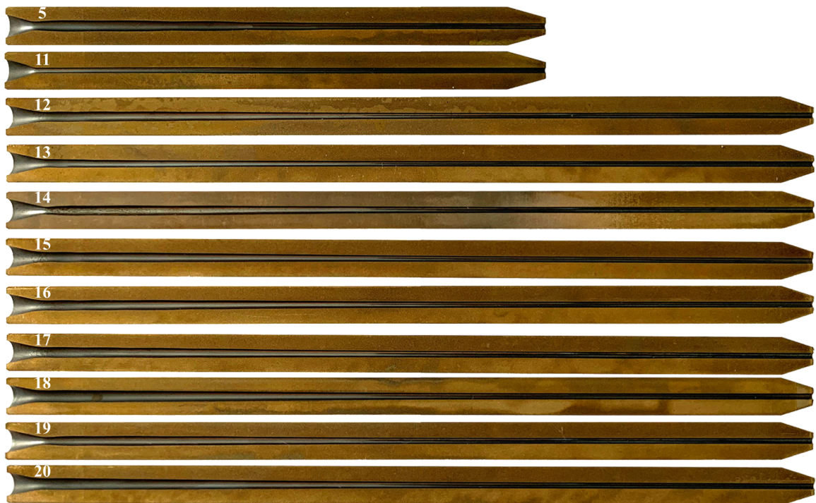
Figure 5.12: Comparison of wear between mixing tubes subjected to regular and accelerated wear using garnet or \text{Al}_2\text{O}_3 abrasives. Tube 5 was worn using accelerated wear, with all other tubes worn using regular wear.
