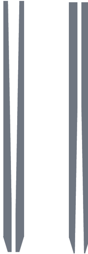
Figure 2.2: Possible wear patterns of AWJ mixing tubes – as observed by Hashish [7]. When using hard abrasives like garnet, a mixing tube made of hard material exhibits a convergent wear pattern, whereas a mixing tube made of soft material exhibits a divergent wear pattern.
