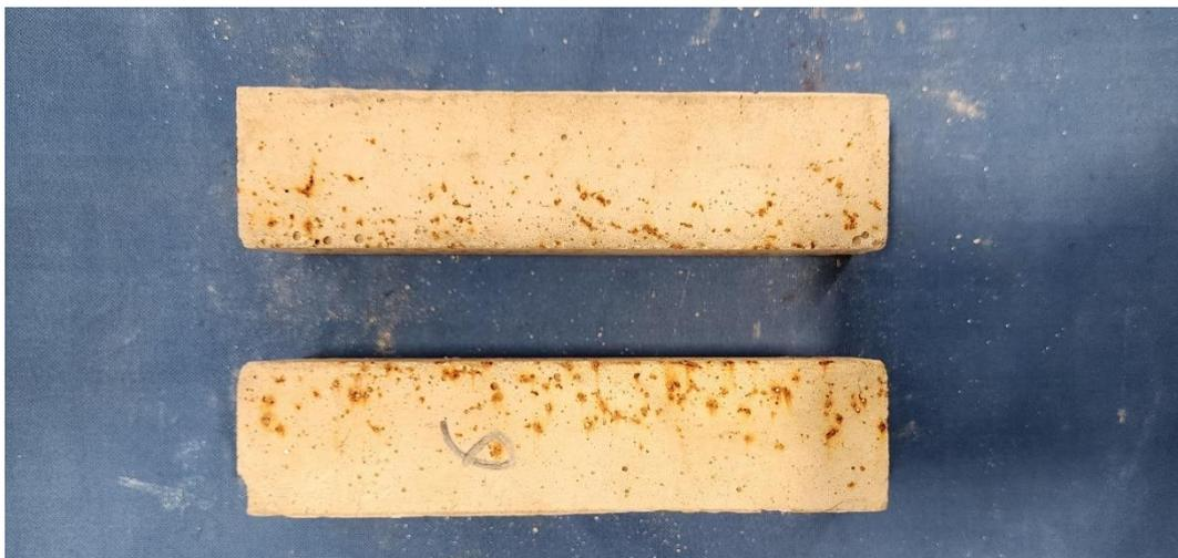
**Figure D.4.1-4 - Side profile SB50M 10MK (4 month corrosion)**
