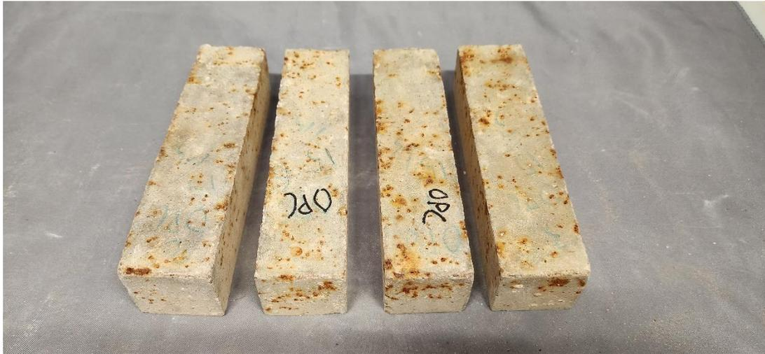
**Figure D.4.1-8 – Corrosion of OPC**
