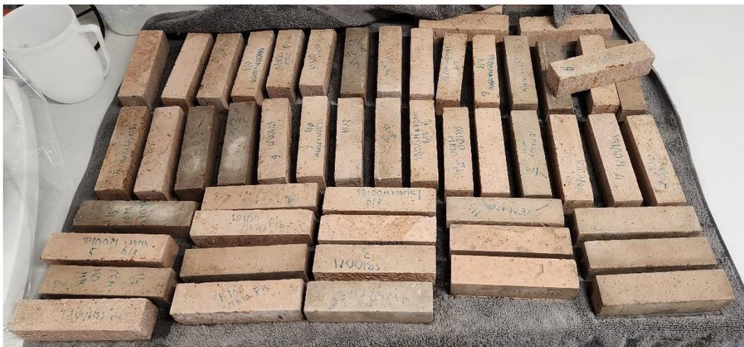
Figure D.4.1-1 –Prisms exposed to corrosion acceleration
