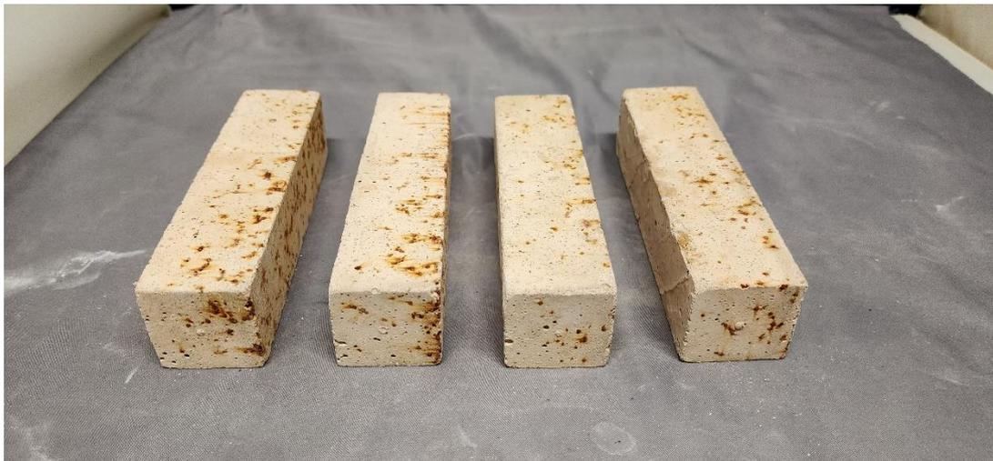
**Figure D.4.1-7 – Corrosion of SB50M 10MK**
