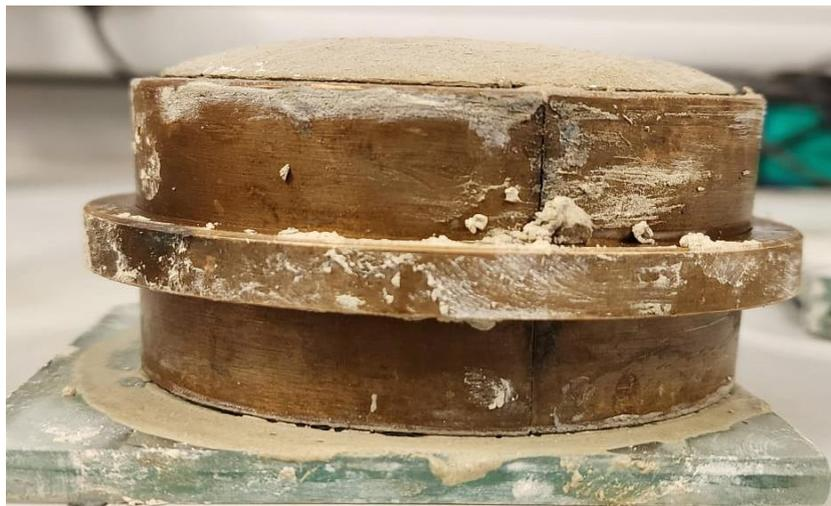
**Figure B.1-1 – SB50L expansion during setting time tests**
