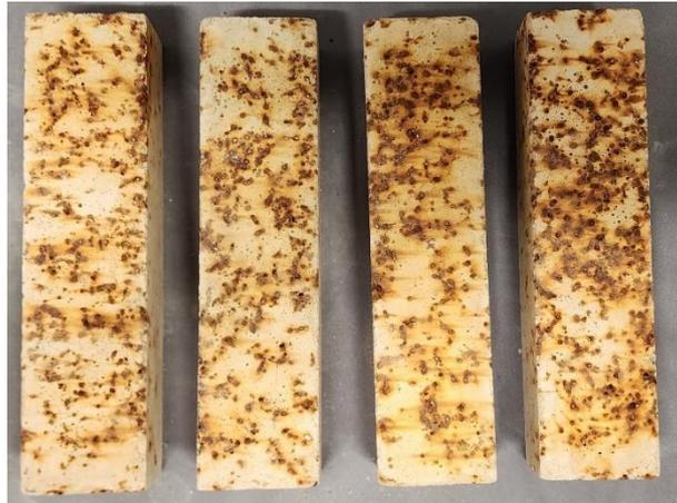
**Figure 6-24 - SB50M following 8 months of corrosion**
