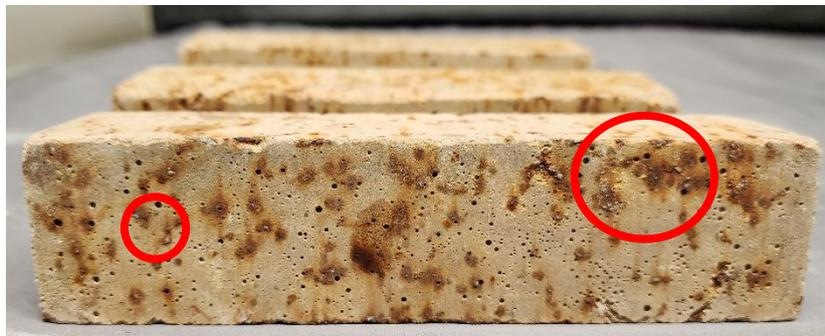
**Figure 6-25 - Fibres exposed likely due to chloride acceleration**
