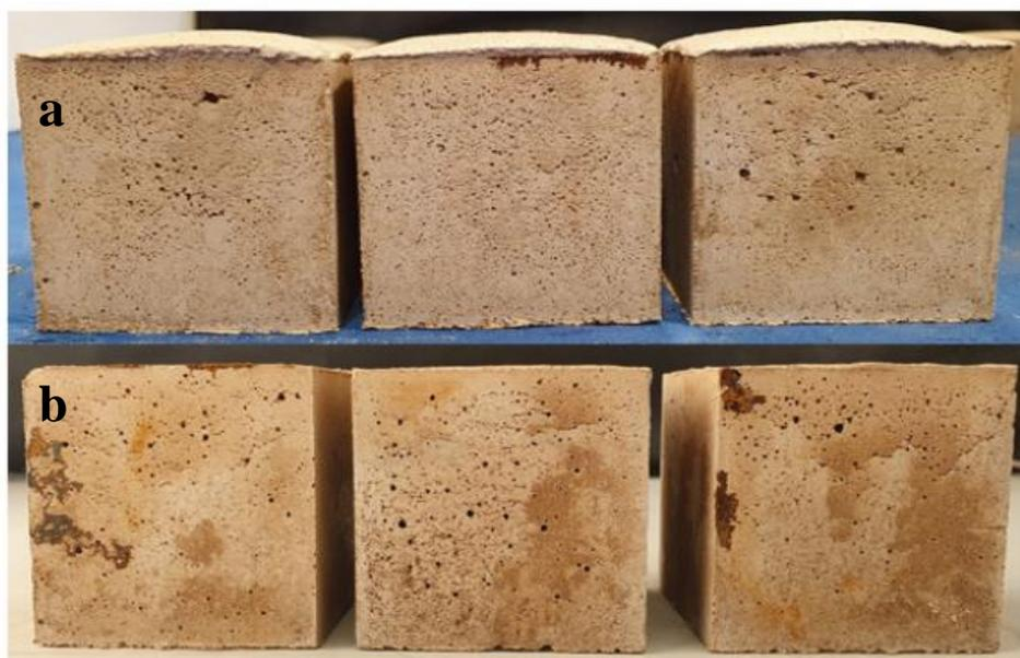
**Figure 3-3 - Side profile of CBPD binders (a) KGH (b) KGA**
