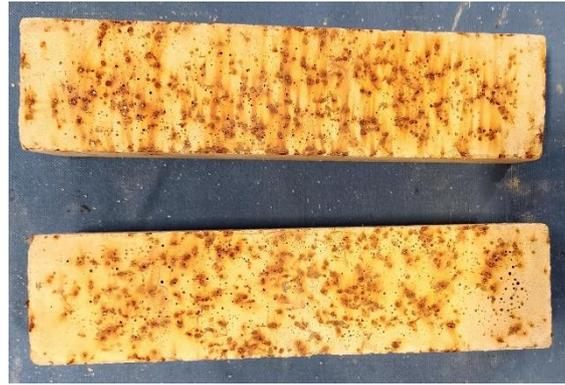
**Figure 6-22 – View of the external corrosion of the prisms**
