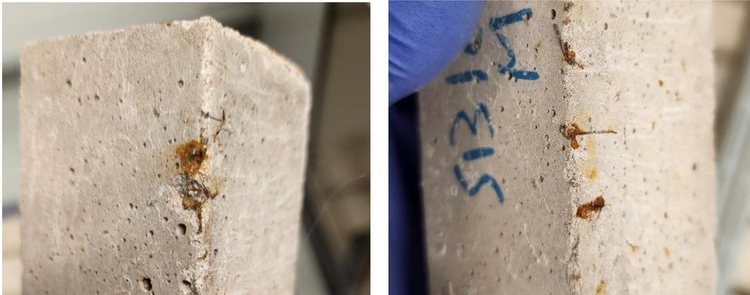
**Figure 6-21 - Minor corrosion due to water curing**
