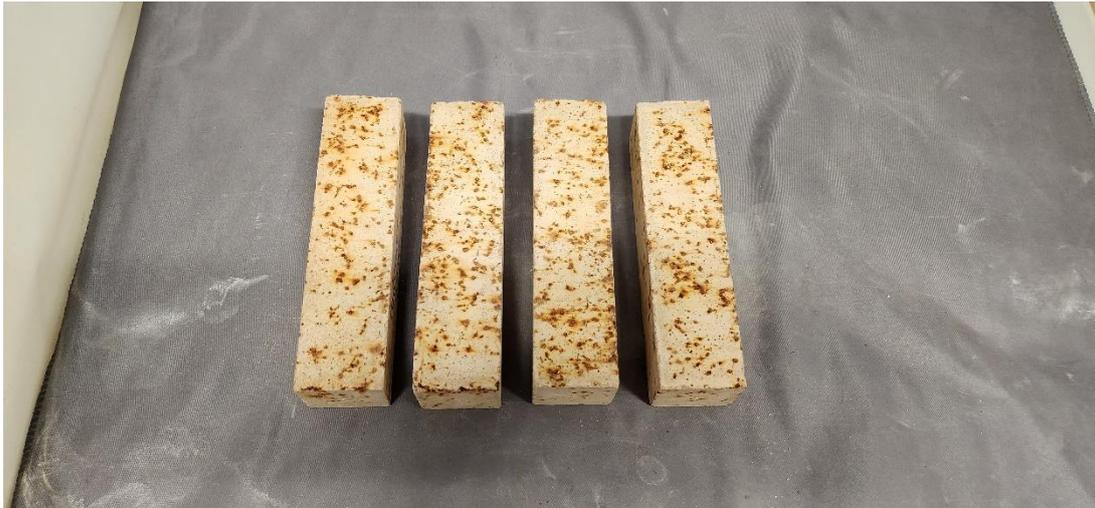
**Figure D.4.1-11 – Corrosion of SB50M**
