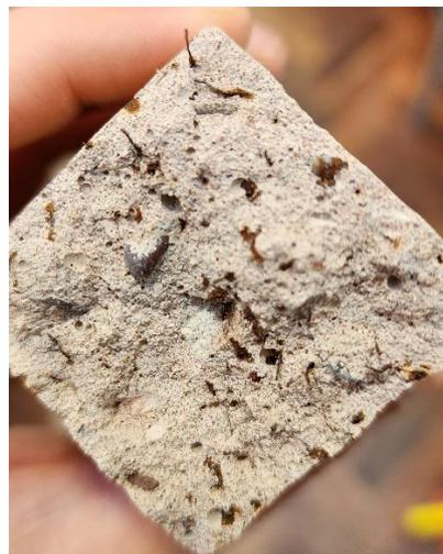
**Figure 6-25 - SB50M showing signs of rust in the centre of the prism**
