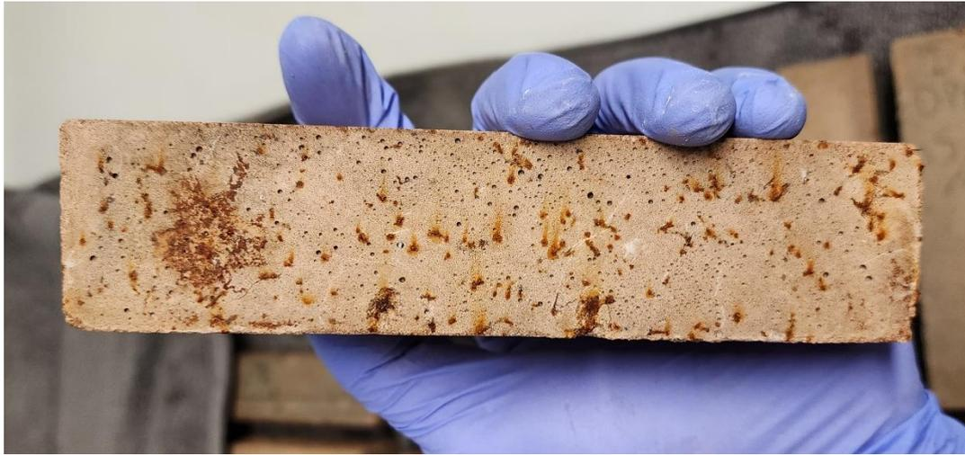
**Figure D.4.1-2 – Agglomeration of corroded fibres**
