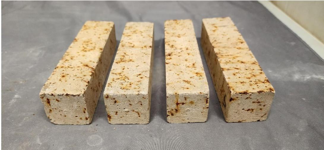
**Figure D.4.1-5 – Corrosion of SB50M 20MK**
