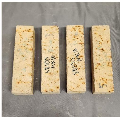
**Figure D.4.1-10 – Corrosion of SB50 10MK**
