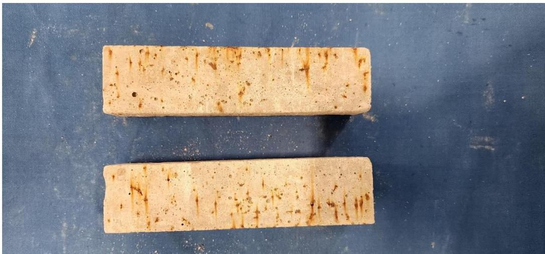
**Figure D.4.1-3 - SB50M 20MK corrosion after 4 months**
