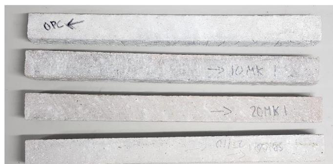
**Figure 6-4 - Bars cast for ASR testing**
