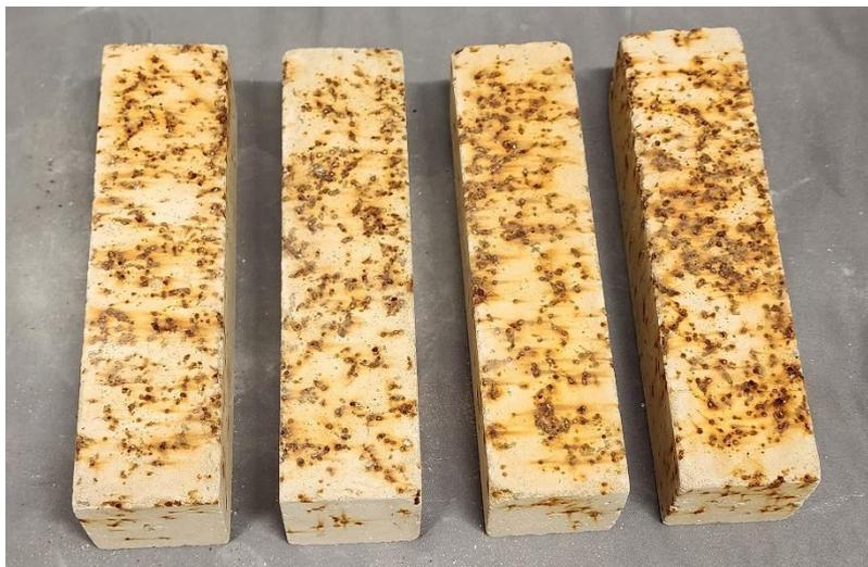
**Figure D.4.1-12 – Corrosion of SB50**
