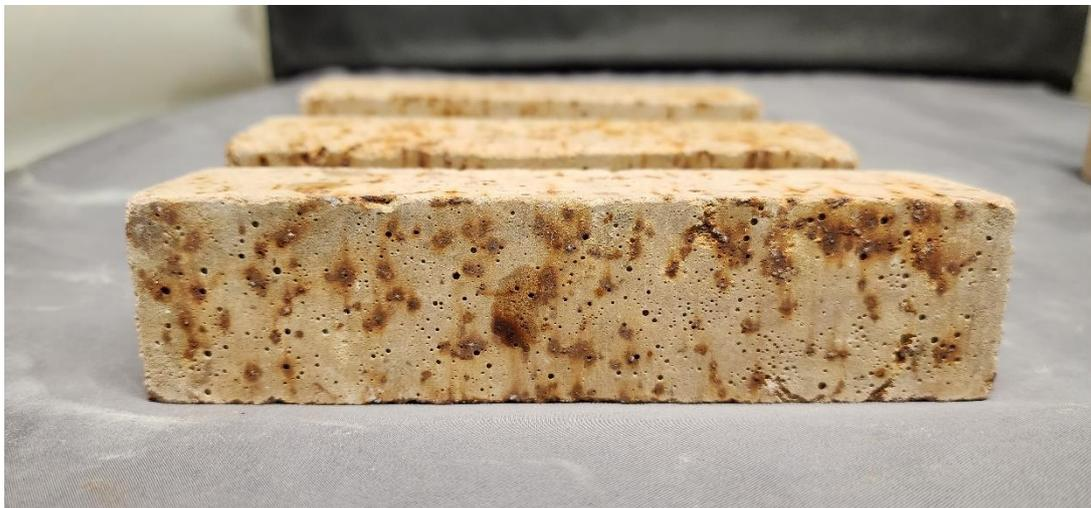
**Figure D.4.1-6 – Corrosion of SB50M**
