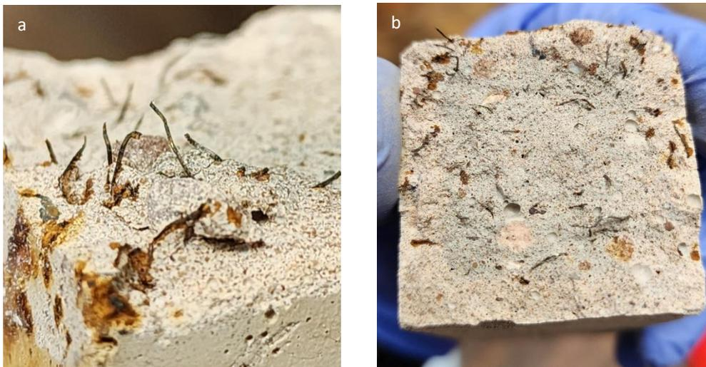
**Figure 6-23 - Corrosion of prisms (a) near surface corrosion of fibres (b) cross-sectional view**
