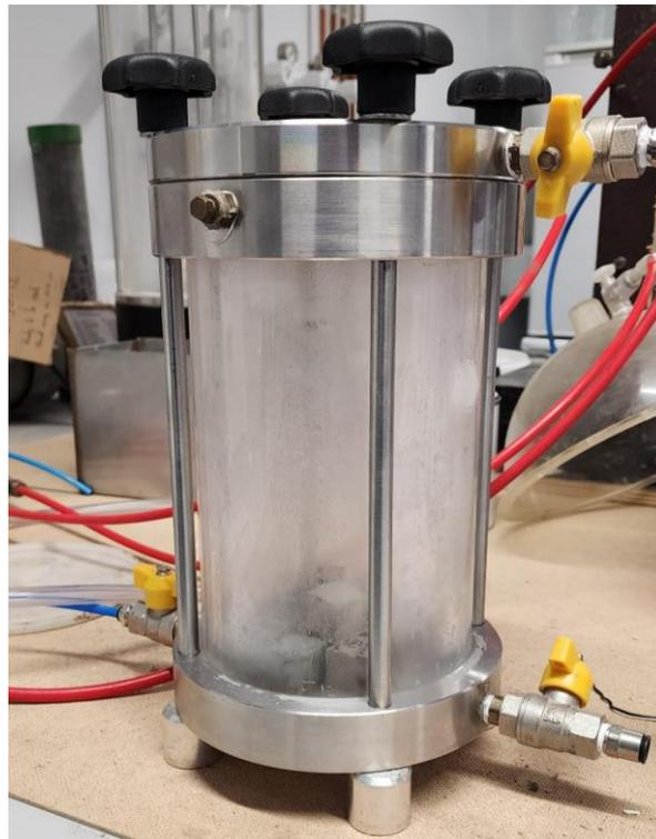
Figure C.1-1 - Carbonation chamber
