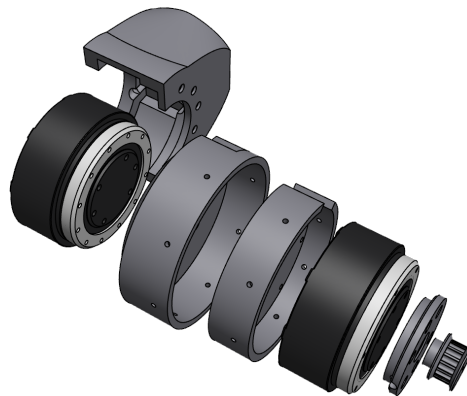
Figure 3.23 Shoulder-Hip joint exploded view. The joint has four 3D printed parts and one pulley.
