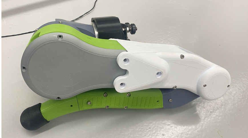
Figure 3.20 A physical leg made by 3D printing.
