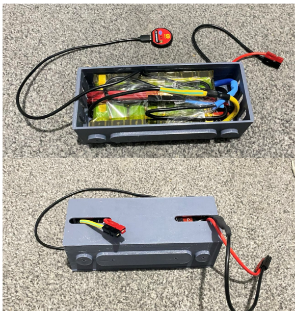
Figure 3.31 Battery module. The top shows the internal battery pack, and the bottom picture is a complete battery module
