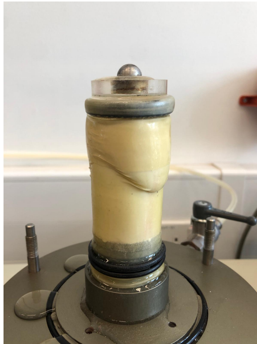
Figure 3.6: Example of evidence of shear failure after triaxial test of kaolin sample consolidated at 400 kPa.
