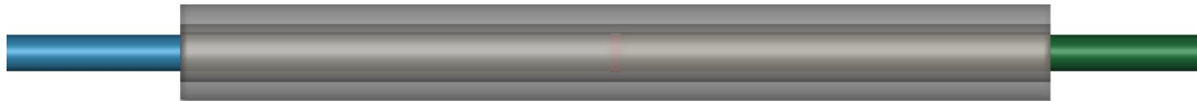
Fig. 17: LS-DYNA cross section zoom-in on the sample inside the partial lateral confinement SHPB set up containing the incident bar (blue), transmitted bar (green), water reservoir (grey), water annulus within reservoir, and the sample (red).
