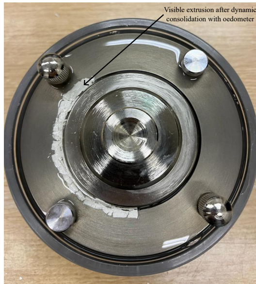
Figure 3.9: Image after kaolin was dynamically consolidated using an oedometer to 3200kPa.
