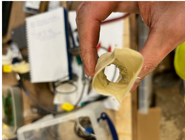
Figure 6.52: Image of kaolin clay sample forming a loop within latex membrane after partial lateral confined SHPB test.
