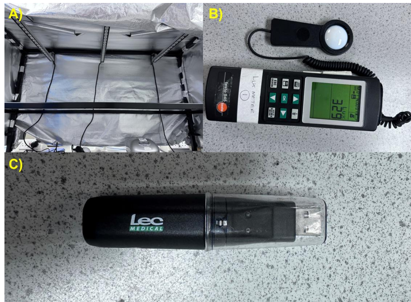
Figure 3.6 A) Growth chamber; B) Testo 545 lux meter; C) Auto-logger.
