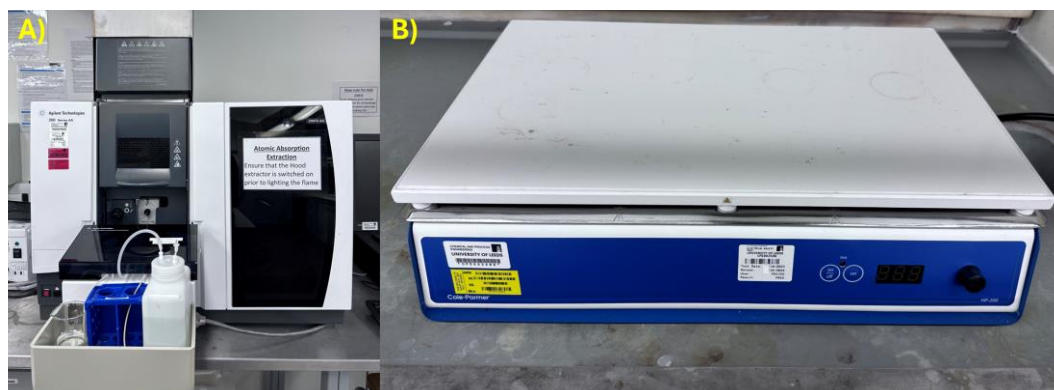
Figure 3.4 A) Atomic absorption spectrophotometer and B) Cole-Parmer HP-200D-XL-C hot plate.
