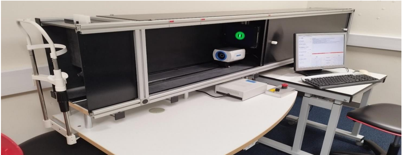
Figure 6. 4 The experimental custom-built apparatus. Participants watched targets displayed on iPad via motorised beam at 4 fixation distances while the PowerRef 3 recorded eye positions and refraction.
