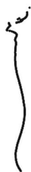
Figure 4.27 The median spline is no longer erratic but contains discontinuities. It cannot be used in subsequent measurements of contour length or curvature.
