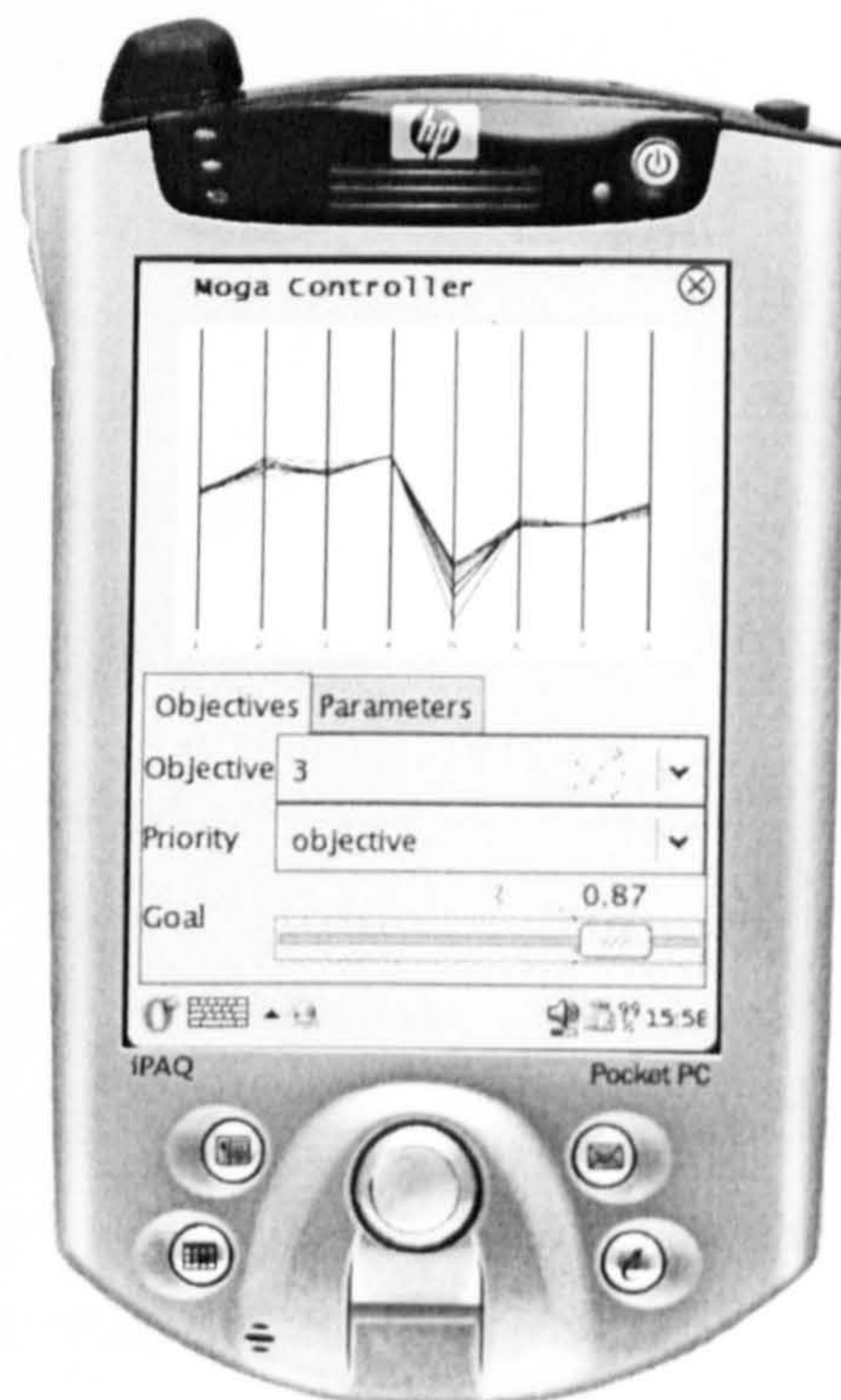
Figure 6.7: A PDA Based Implementation of the Steering Client for a Multi-Objective Evolutionary Algorithm
