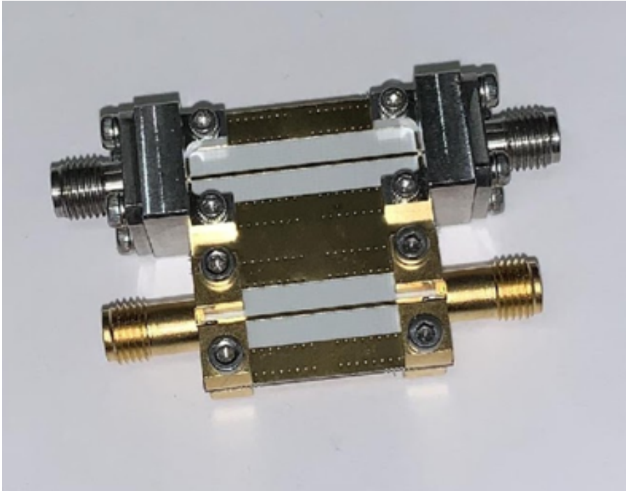
Figure 4.41: Image of the microstrip test boards with both the air core WithWave 2.92mm connector (top) and the PTFE core Rosenberger SMA connector (bottom).
