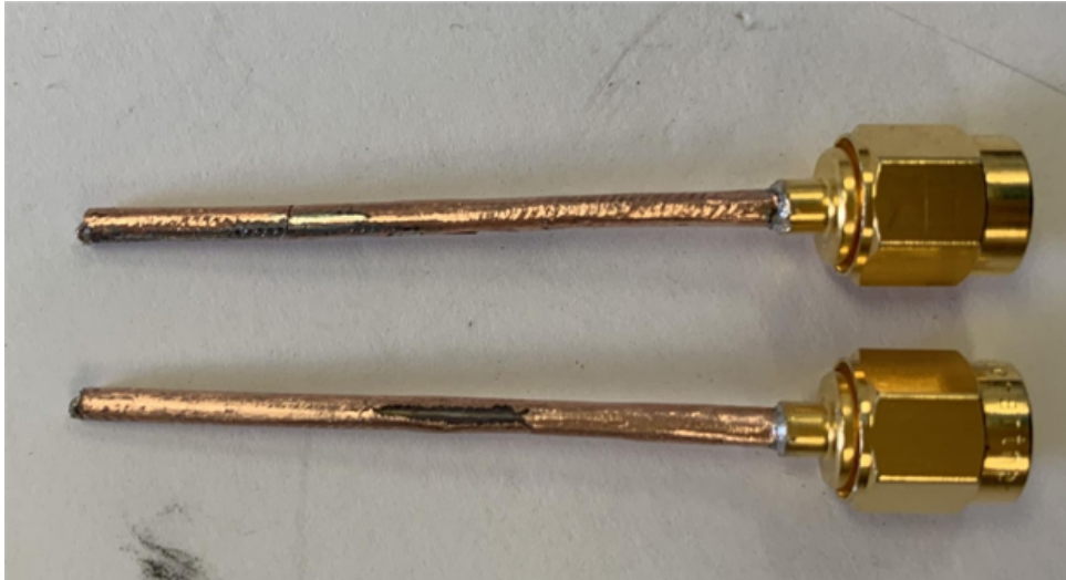
Figure 4.14: Manufactured 'identical' probes. These updated probes were manufactured by hand so they cannot be perfectly identical.
